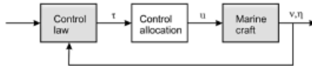
FIGURE 2.6: Block diagram showing control allocation in feedback system [7]
