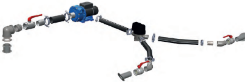
FIGURE 2.3: Exploded view of JT-30 compact system [13]
