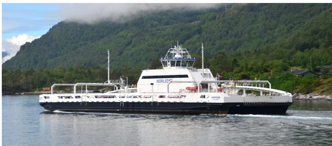
Figure 14: Ampere Electric-Powered ferry
