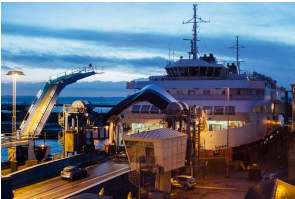
Figure 16: Tycho Brahe: world's largest emission-free electric ferry with the first automated shore-side charging station ( www.abb.com )
