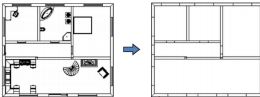
Figure 3.7: Semantic filtering of IFC data (left original model; right only IFCSLAB, IFCWALL, IFCBEAM) (Geiger et al., 2015)
