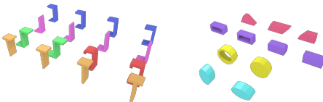
Figure 2.22: IFC parametric curve profiles: (left) those based on the characters U, L, Z, C and T; (right) those based on trapezia, (rounded) rectangles, circles with/without holes and ellipses (Arroyo Otori et al., 2017)
