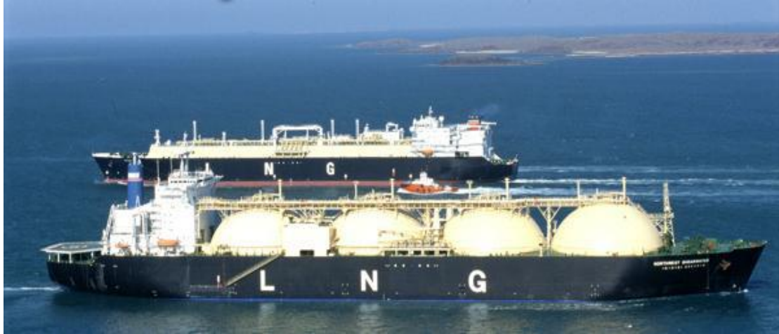
Picture 3 Comparison of a Moss-type and a Membrane type LNG Carrier [3]
