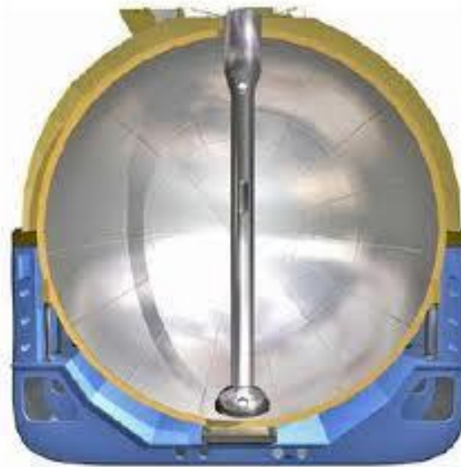
Picture 4 Interior of a Moss Type LNG tank [3]
