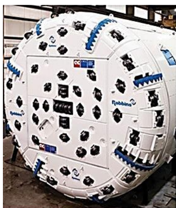
Hard rock TBM
