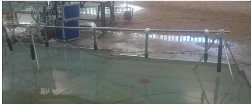
Figure 2 : Layout with vertical quay wall (simulated with smooth iron plate )
