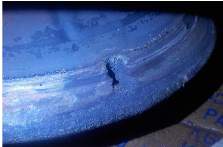
Figure 44: Photo of damage on exhaust valve spindle of Cylinders No.5
