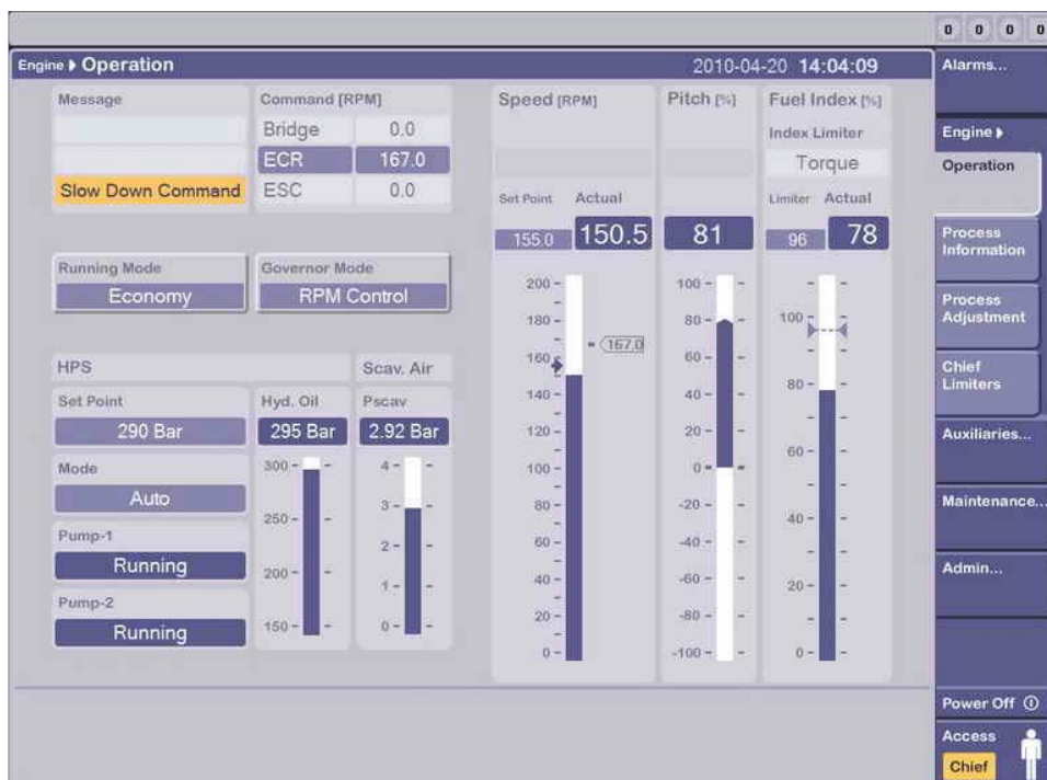
Figure 6.1: Main Operating Panel (MOP) Engine Operation screen [17]
