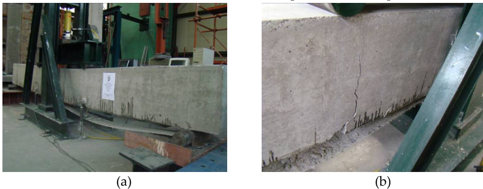
Figure 12: Specimen 2: (a): Debonding along the length of beam; (b): Flexural cracks at mid-span
