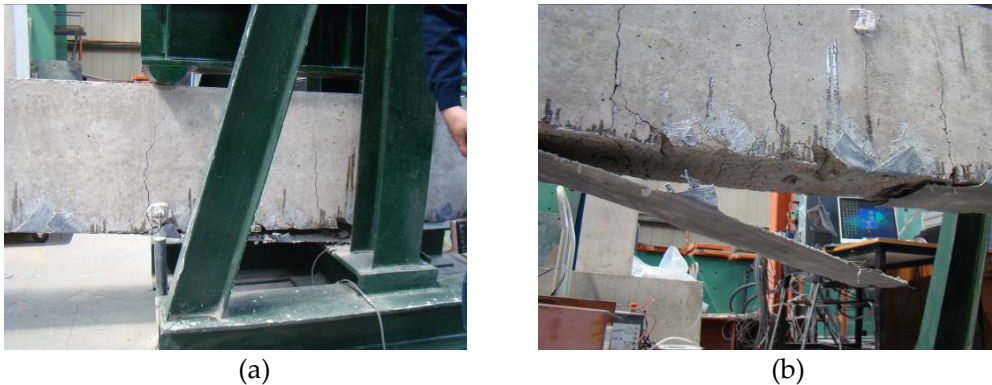
Figure 14: Specimen 3: (a); (b): Flexural cracks at mid-span, rupture of carbon strengthening system
