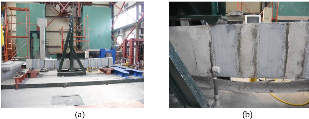
Figure 16: Specimen 4: (a); (b): Debonding of strengthening system
