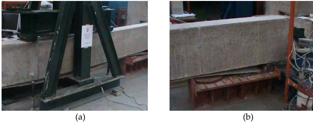
Figure 10: Specimen 1: (a); (b): Debonding of strengthening system at the end of the test
