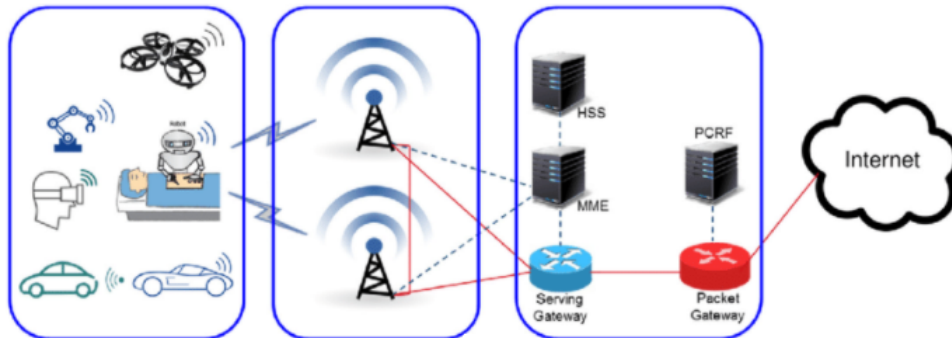
Σχήμα 1.1: 4G υποδομή (MME:Mobility Management Entity, HSS:Home Subscriber Server, PCRF:Policy and Charging Rules Function)
