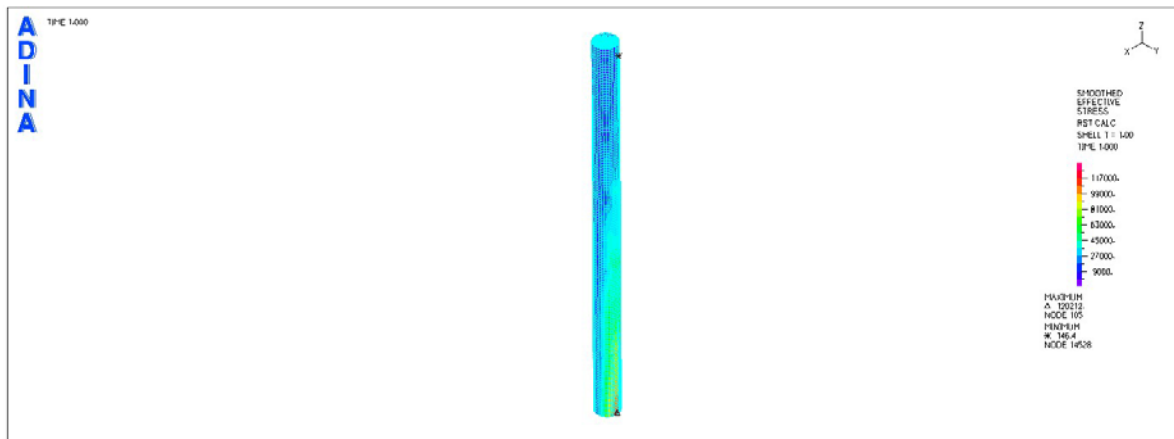
Figure 16: Analysis results for the static stimulant with shell finite elements for the seismic load combination. von Mises stress = 120.212 MPa
