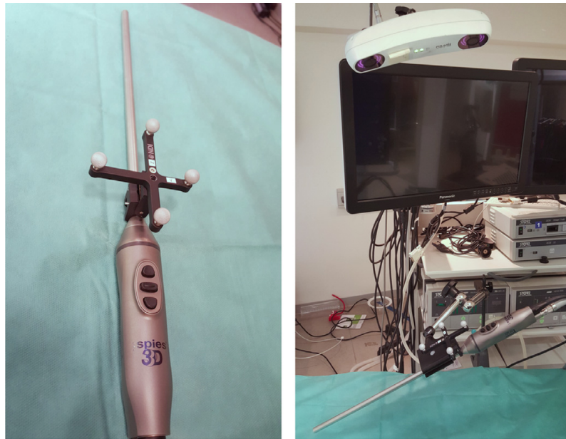
Figure 7.2: A fixed markers pattern placed on the laparoscope for optical tracking and the detection cameras [7].
