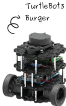
Figure 6.4: The TurtleBot3 Burger differential drive robot. The robot offers an open-source simulation environment with ROS packages and Gazebo support.
