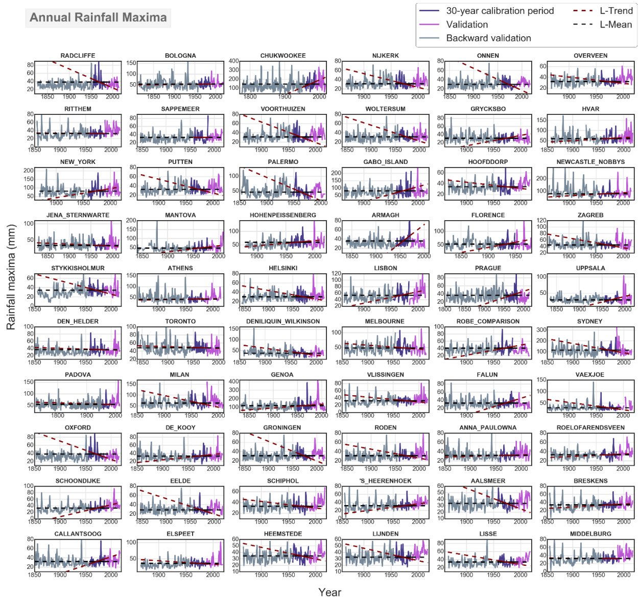
Figure B.5 Local trend vs the local mean in projecting annual maxima for the 60 longest rainfall stations.
