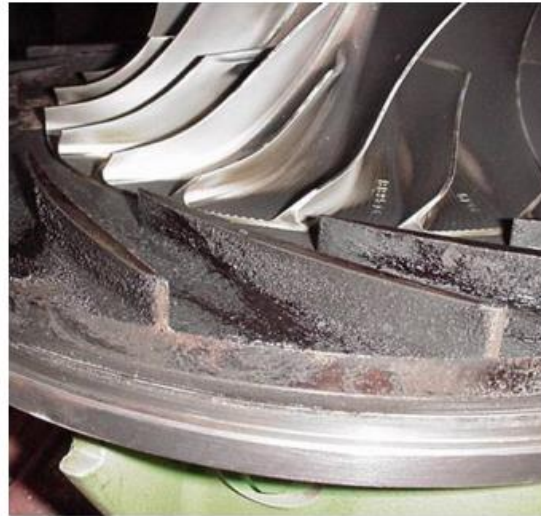
Figure 10: Compressor diffuser with initial carbonization [1]
