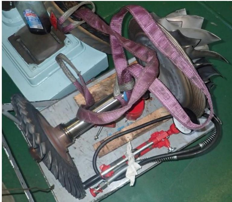
Figure 13: Compressor, Turbine wheel and their shaft taken out for overhauling
