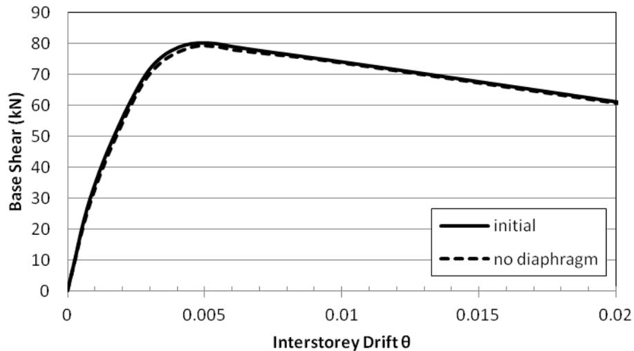
Figure 5–3: Influence of rigid diaphragm (X direction)
