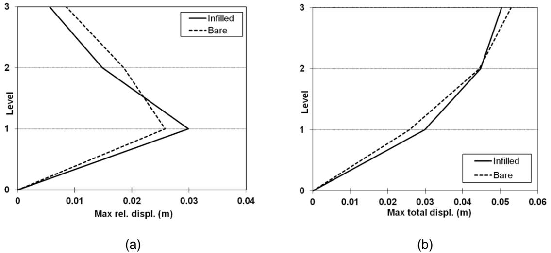
Figure 5–13: Influence of infill walls: (a) Maximum relative displacements (b) Peak shifts
