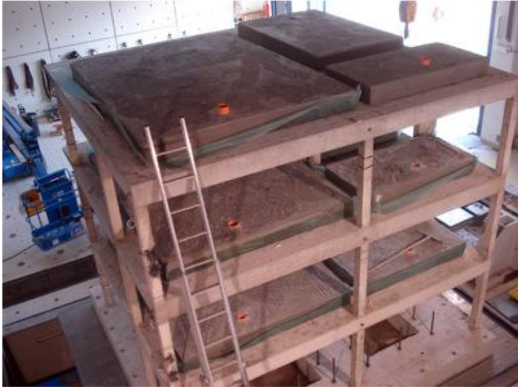
Figure 2–7: Additional mass for the simulation of storey superimposed dead and live loads
