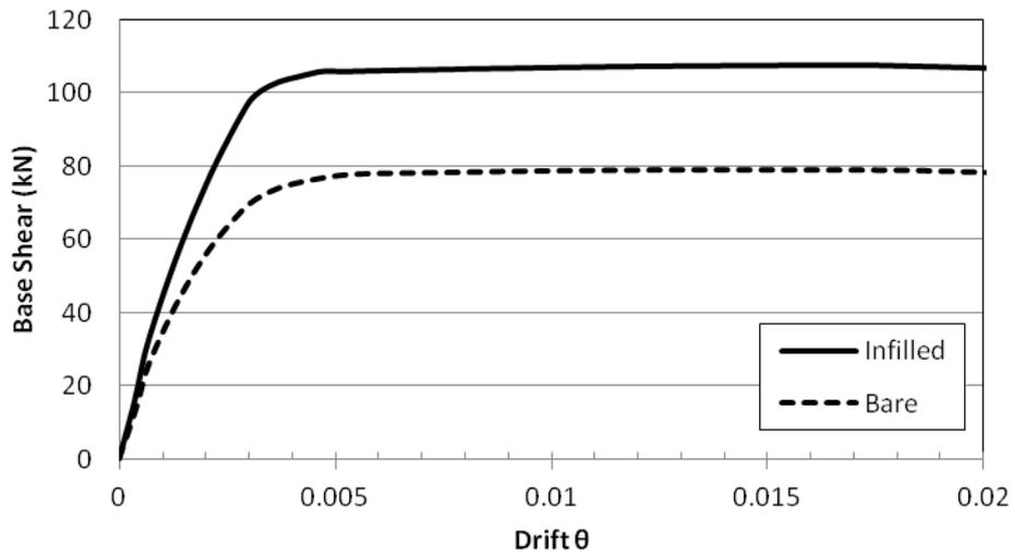
Figure 5-6: Infill walls influence at Y axis
