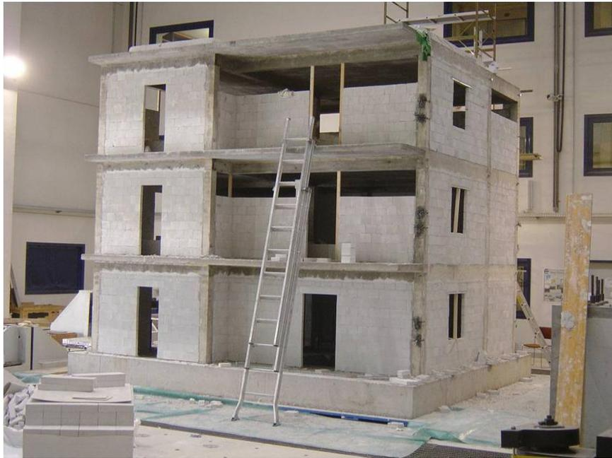
Figure 6–7 Construction of the infill walls
