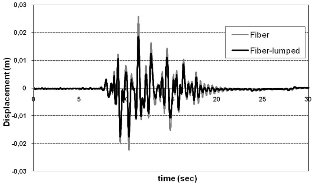
Figure 5–34: Comparison, in pairs, of 1<sup>st</sup> floor displacement time histories for the three different simulations
