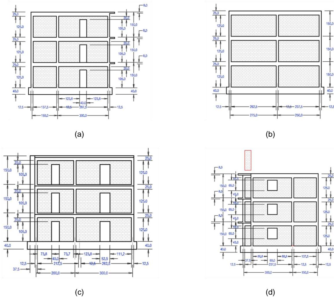
Figure A-4: Construction of walls (a) A, (b) B, (c) C, (d) D view
