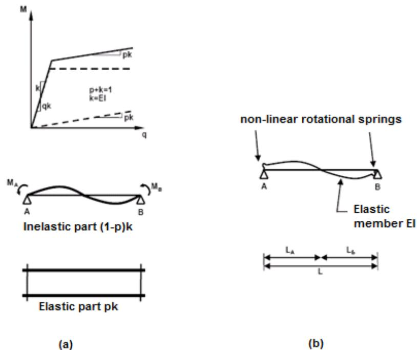
Figure 3–9: Simplified item with concentrated plasticity (a) Model of Clough-Johnston (b) Model of Giberson
