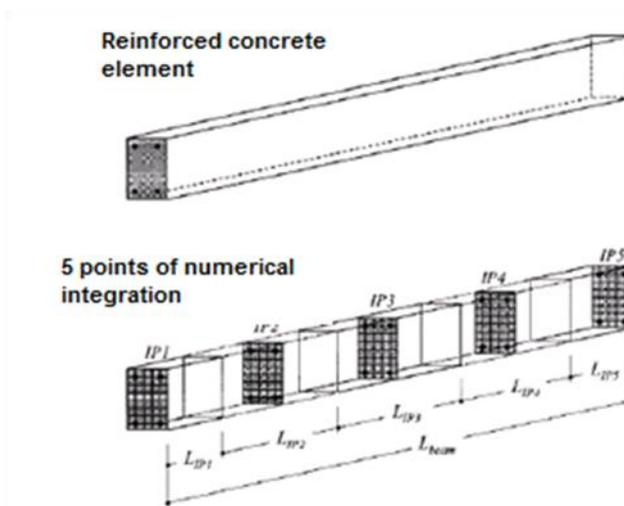
Figure 3–8 Beam element with five-point numerical integration
