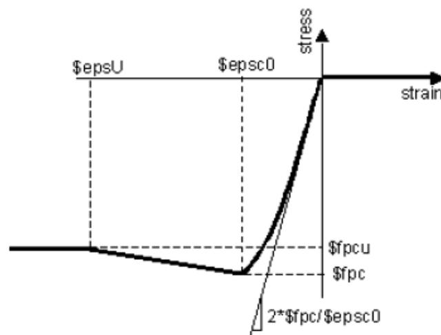
Figure 3–16 Trend Chart model "Concrete01" deformation under monotonic loading
