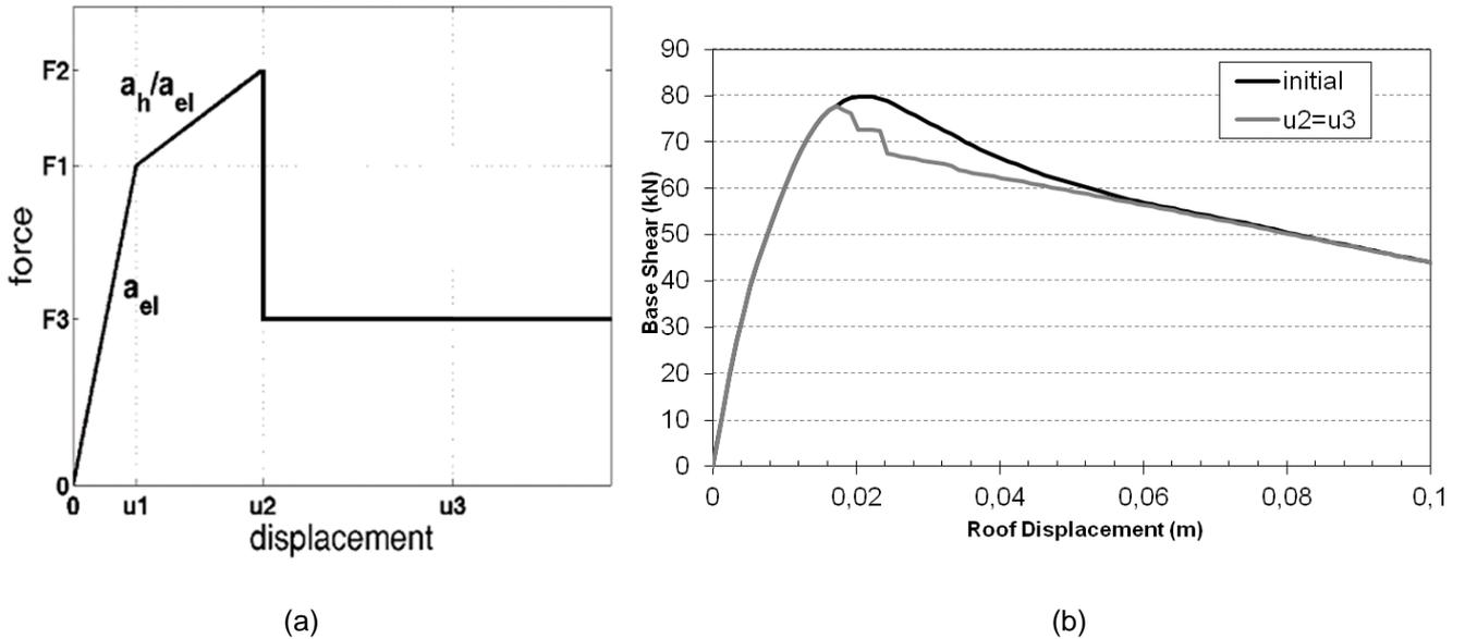
Figure 6-9 (a) Second hypothetical model ( $u_2 = u_3$ ) and (b) the response of the building respectively
