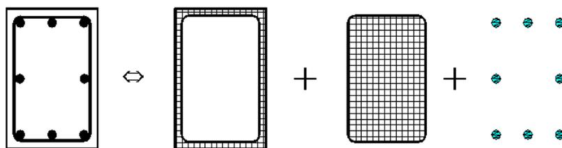
Figure 3–3 Simulation of the reinforcement concrete section with force-based elements
