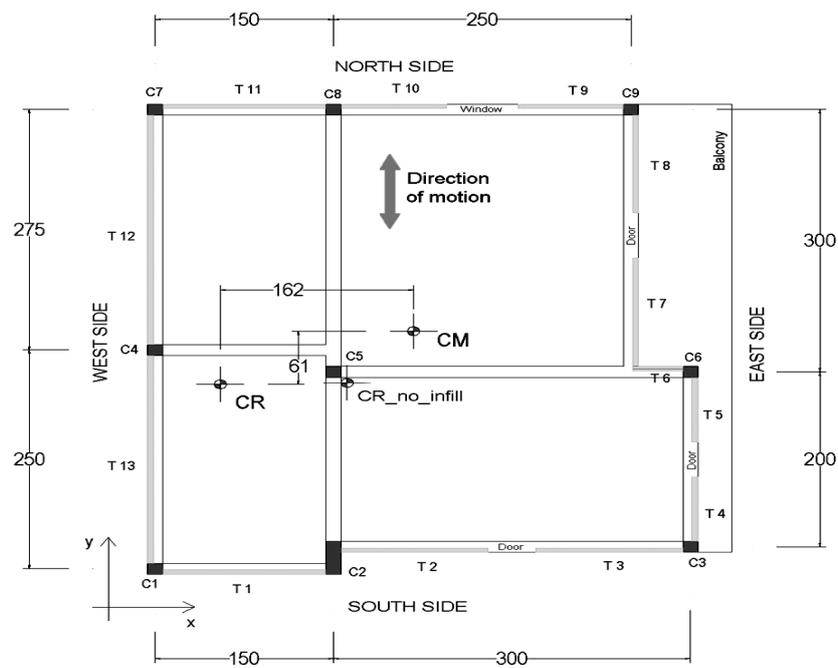
Figure 5-30: Typical floor plan
