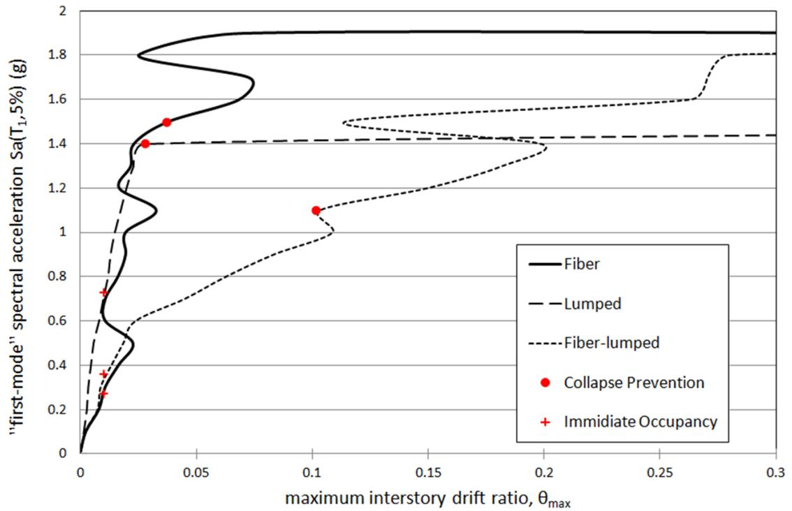
Figure 7-6 Median IDA curves for the three different elements
