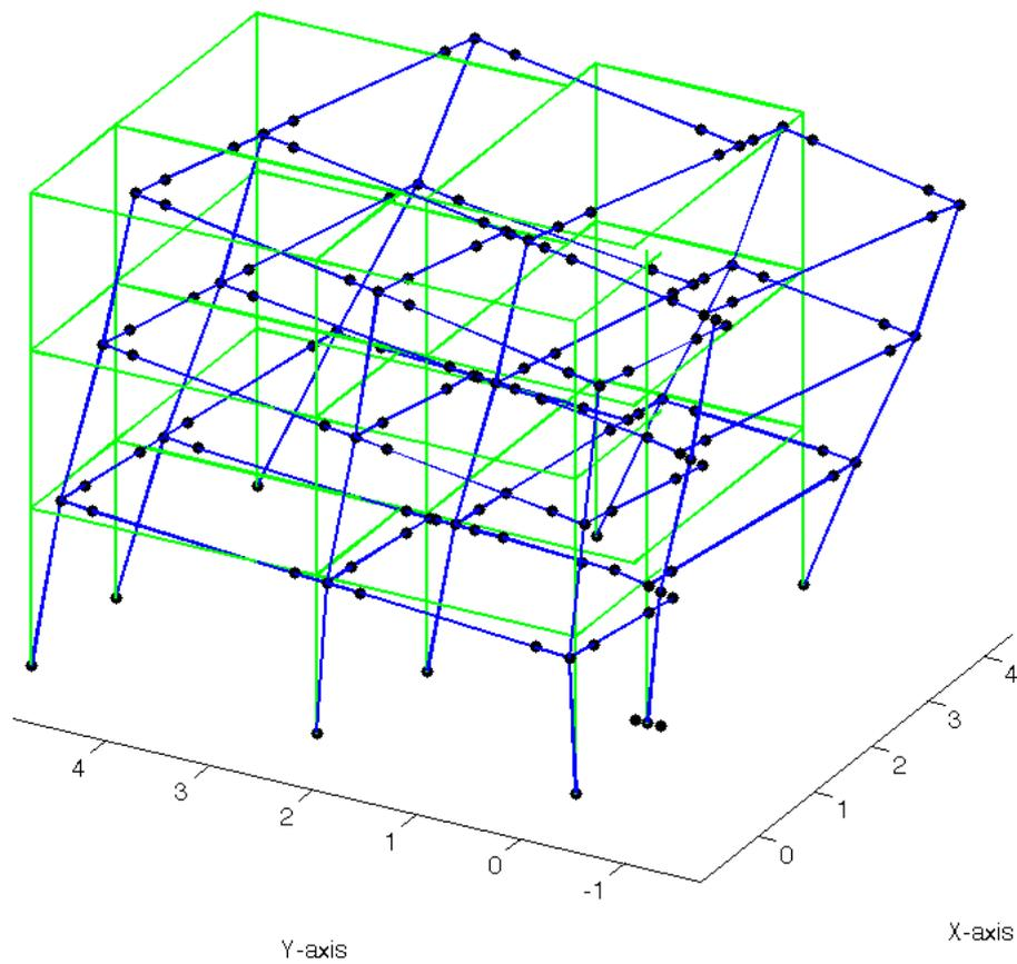
Figure 4-2 Display of 1<sup>st</sup> Eigenperiod
