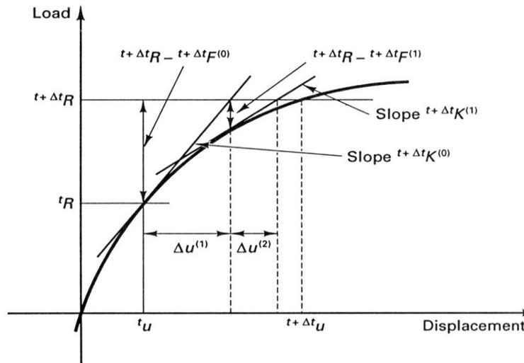
Figure 3-2 Schematic illustration of the method of Newton-Raphson
