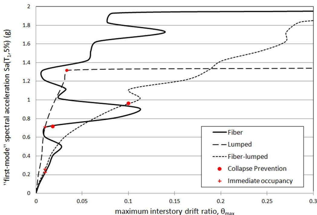
Figure 7-5 IDA curves for the sakaria records, three different elements
