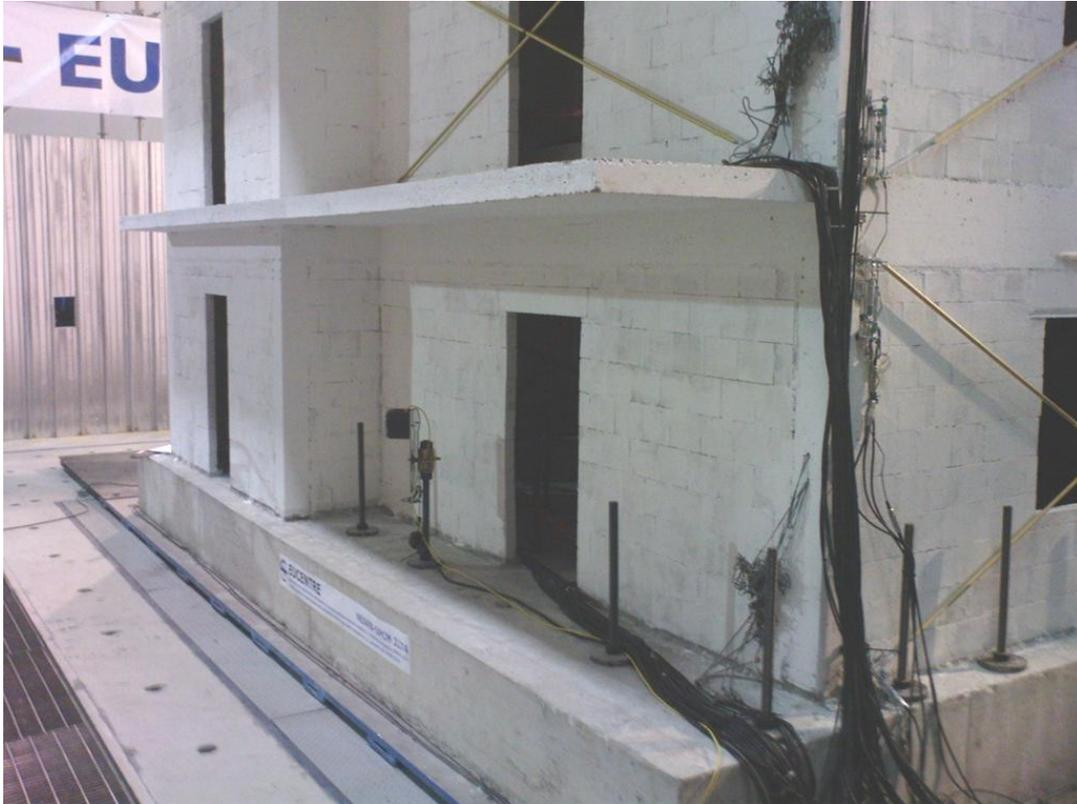
Figure 5–9: Displacement gauges of column C6
