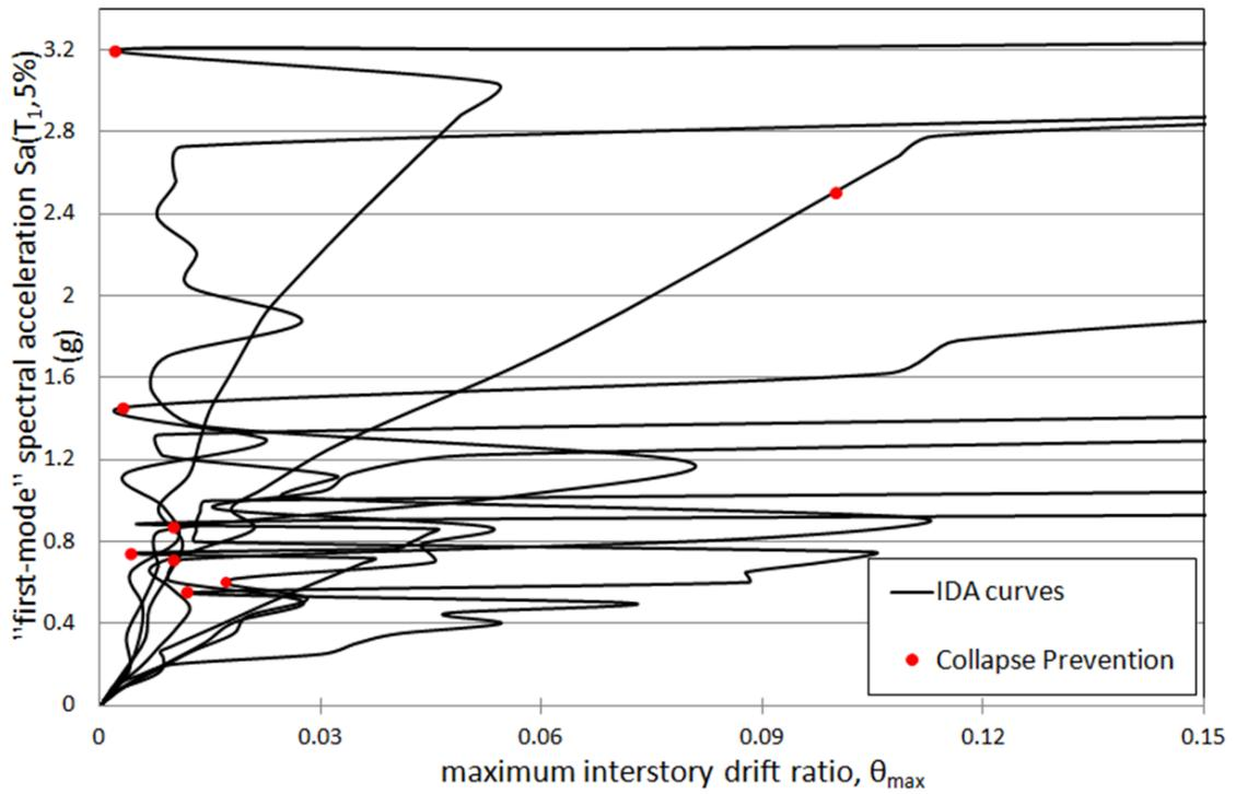
Figure 7-3 All eight IDA curves and the associated limit-state capacities. The IO limit is at the intersection of each IDA with the  $\theta_{\max}=1\%$  line, the CP limit is represented by the dots.
