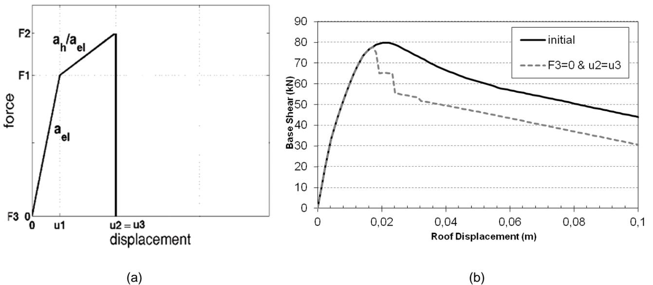
Figure 6-10 (a) Third hypothetical model ( $u_2 = u_3$  &  $F_3=0$ ) and (b) the response of the building respectively
