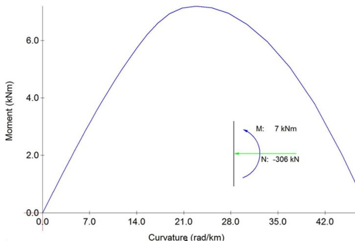
Figure 3–12 Bending curve for axial load N=306kN
