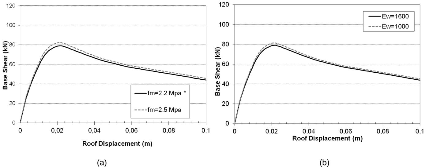
Figure 6–6 Response of the structure depending on the rate of variation in (a)  $f_m$ , (b)  $E_w$
