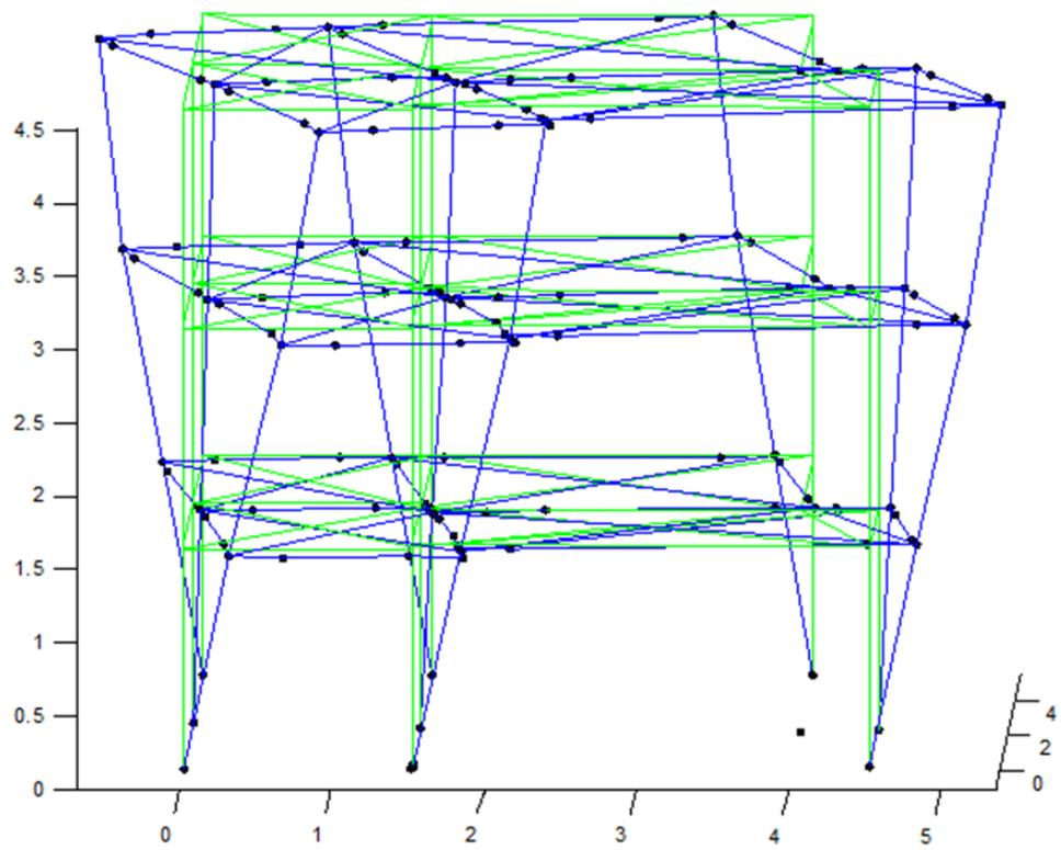
Figure 4-4 Display of 3<sup>rd</sup> Eigenperiod
