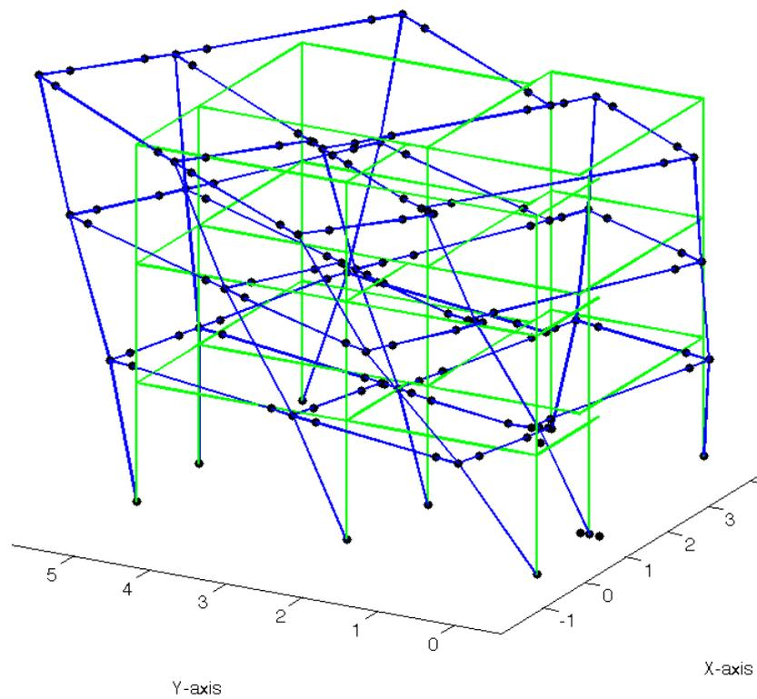
Figure 4-3 Display of 2<sup>nd</sup> Eigenperiod
