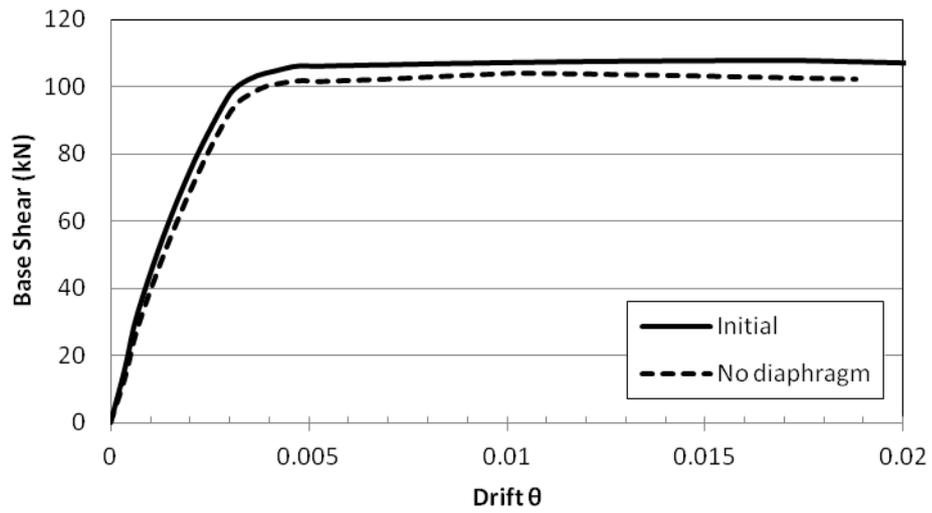
Figure 5-7: Slab stiffness influence at Y axis
