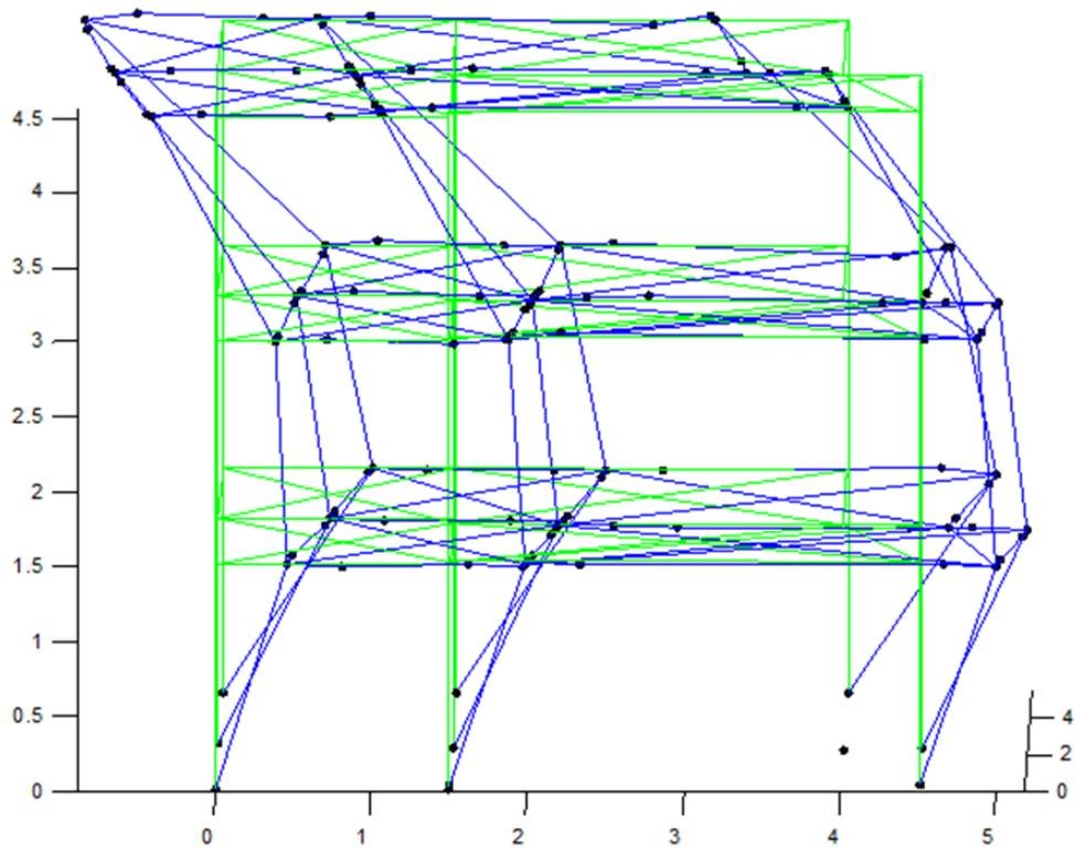
Figure 4-5 Display of 4<sup>th</sup> Eigenperiod
