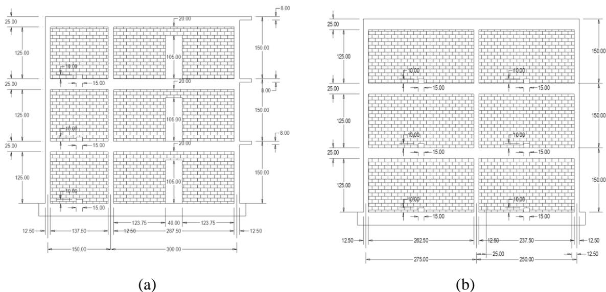
Figure 2–3: Side frame elevations: (a) view A-A, (b) view B-B (see notation of Fig. 2 -2)
