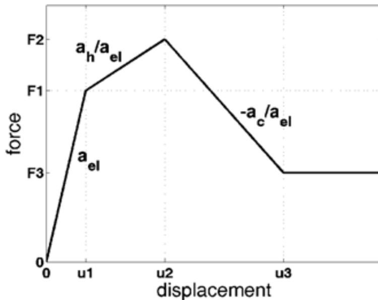
Figure 6-1: Quadrilinear peak-oriented model used for modeling the masonry infills
