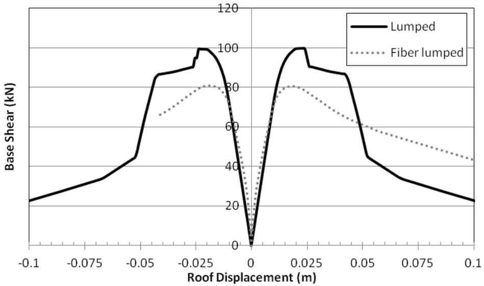
Figure 5–25: Comparison of simulation between lumped and fiber lumped elements on X axis
