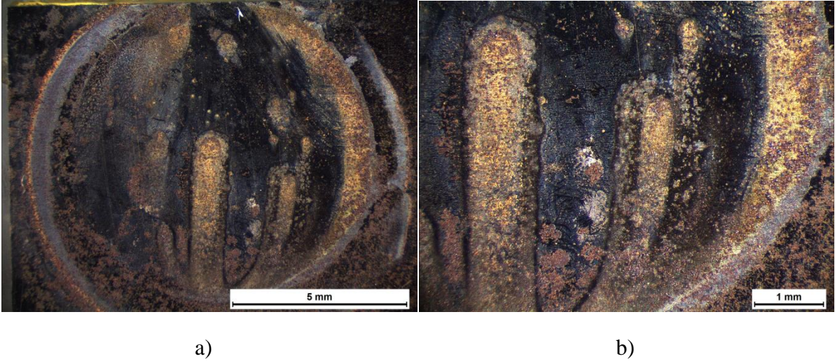
Fig.[12.5] Optical observation of parent metal AH36 after the first series of Electrochemical Impedance Spectroscopy a) x1.0, b) x2.0.
