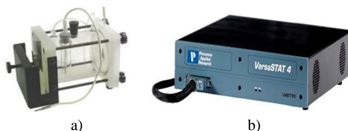
Fig.[5.4] a) Three-electrode electrochemical cell, b) VersaStat 4 potentiostat.
