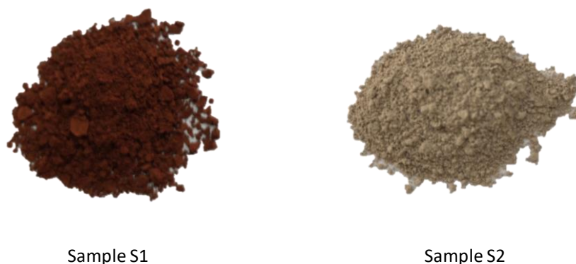
Figure 31 Solid residues after leaching. The reddish one (Sample S1) is from the dissolution of BR at 150 °C, 200 rpm, 5% w/v pulp density for 24 h and the greyish one (Sample S2) is from the dissolution of BR at optimum conditions.
