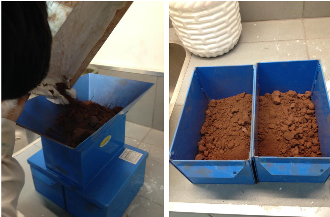
Figure 11 The Jones riffle splitter present at NTUA laboratory.
