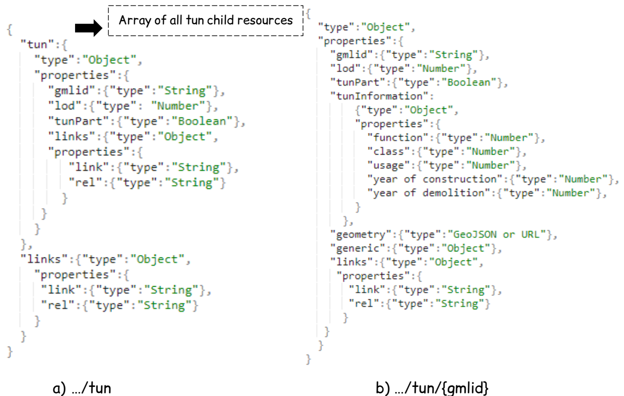
Figure 4-24: JSON-based tun resource schema
