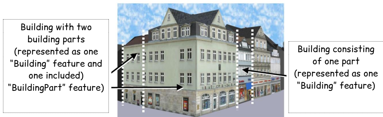
Figure 4-3: Examples of building consisting of one and two building parts
