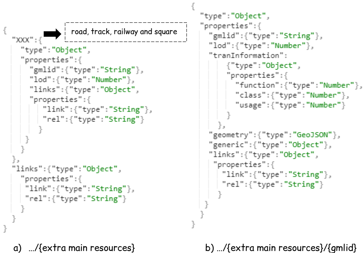
Figure 5-18: JSON-based schema of extra main resources (road, track, railway and square)
