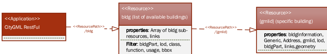
Figure 4-4: Conceptual design of the "bldg" main resource
