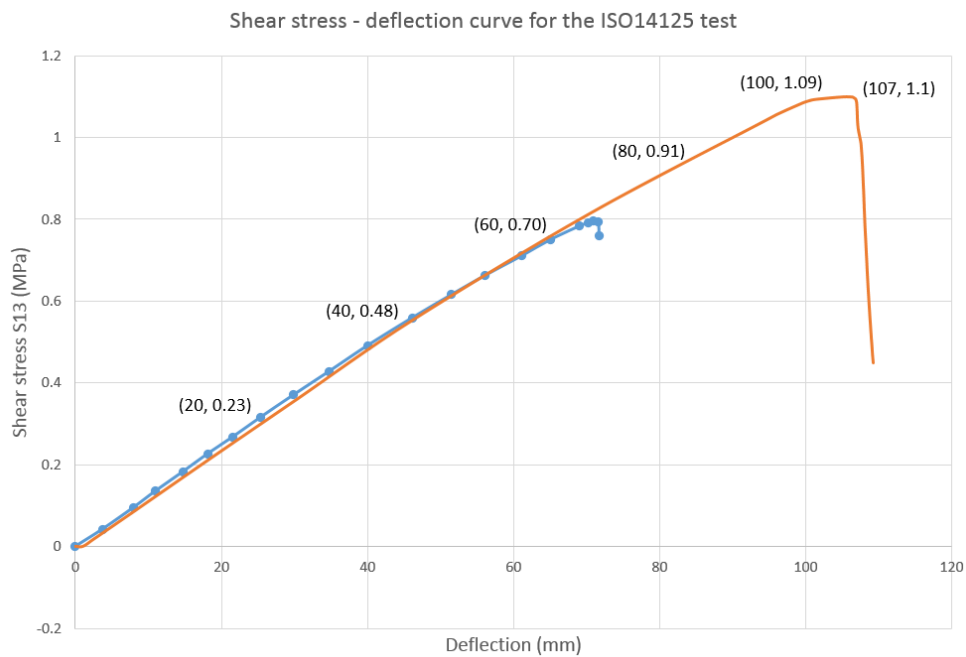
Figure 4.10: Difference in the maximum deflection where failure occurs between modeling and experiment
