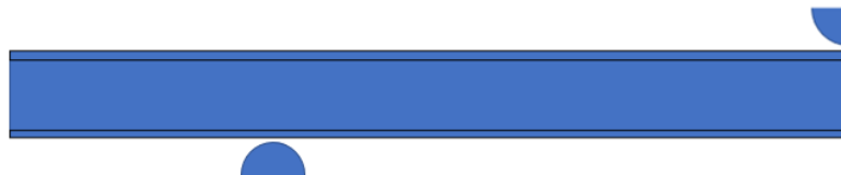
Figure 3.2: Modeled geometry of the 3-point bending test
