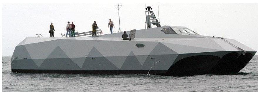
Figure 1.3 M80 Stiletto naval ship made of carbon fiber composite
