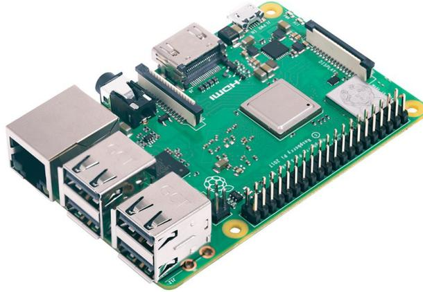
Figure 29: Raspberry pi 3 model B+ - The Central Control Module (CCM)
