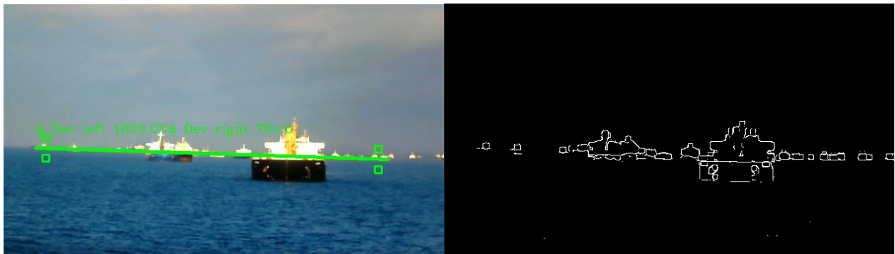
Figure 4.7.1 Images of horizon line detected using square windows to compare the two different areas of sky and sea. It is also written the deviation values computed in each side of the line. In the right the computed finale-edge map from which the lines where computed is shown.
