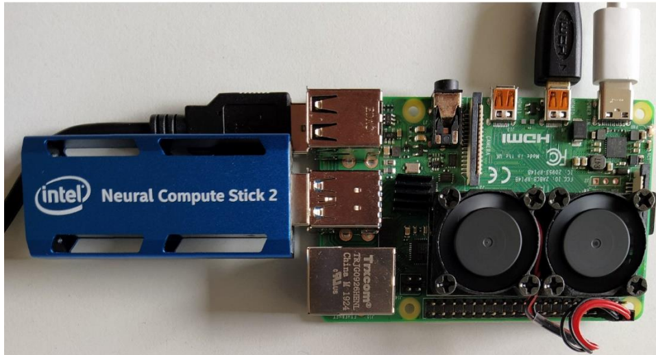
Figure 2.3 Presents our hardware computational selection, comprises of Raspberry Pi4 as the main system control board and the Intel Neural Compute Stick2 which executes our deep neural network
