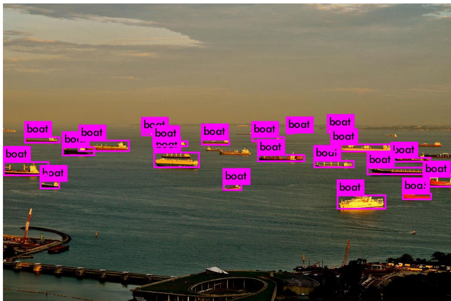
Figure 3.18 a) An image of a busy port and the detected Sea-Vessels within the boat annotated boxes
