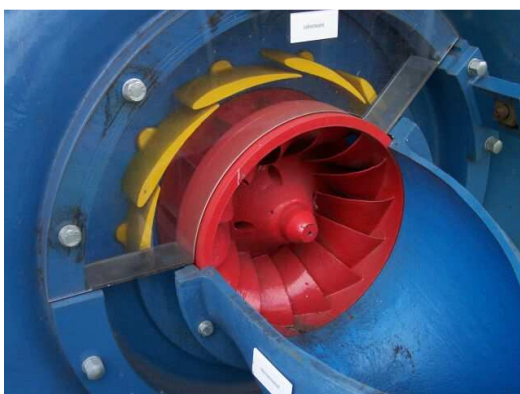
Cut-away view, with guide vanes (yellow) at minimum flow setting
