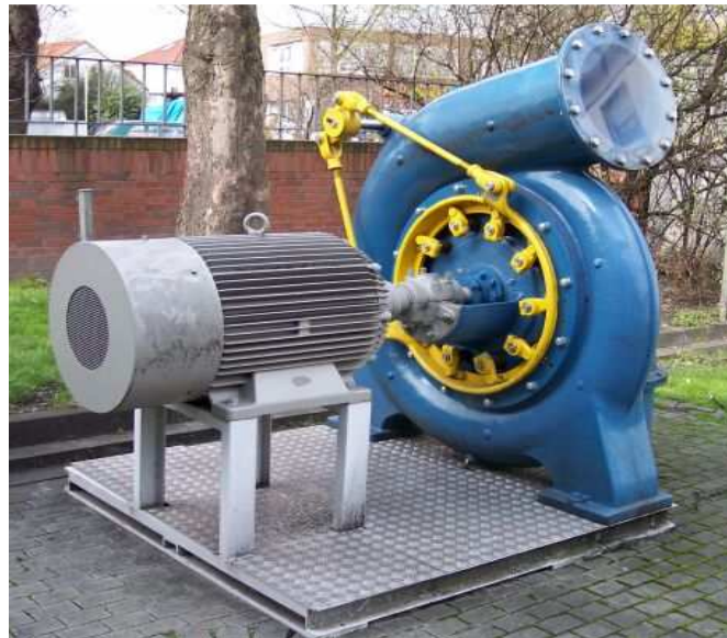
Francis Turbine attached to a generator
