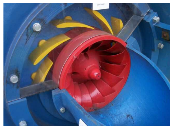
Cut-away view, with guide vanes (yellow) at full flow setting
