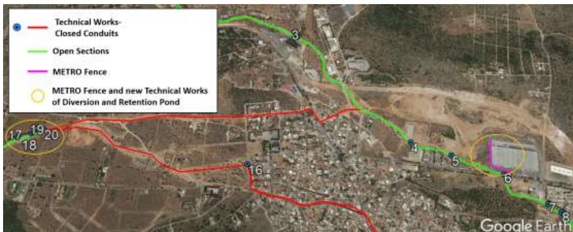
Figure 26 New technical works of diversion and retention pond (Scenario “Diversion, retention pond and METRO fence”)
