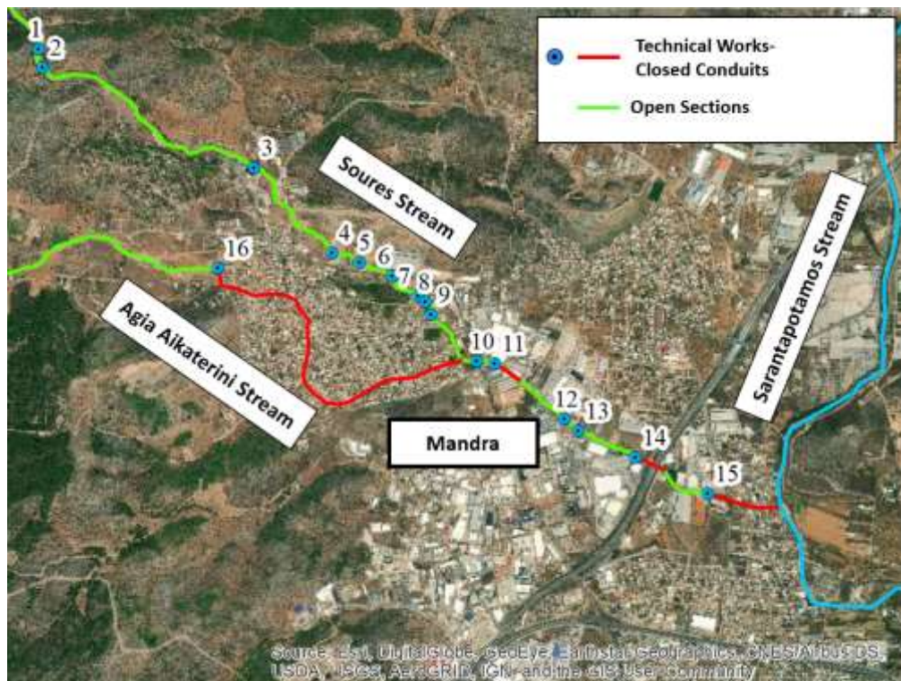
Figure 2 The town of Mandra with the hydrographic network and technical works
