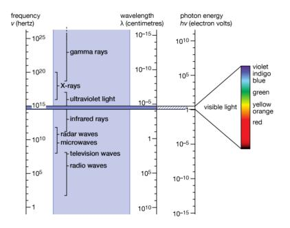
Figure taken from [3] displays the electromagnetic spectrum
