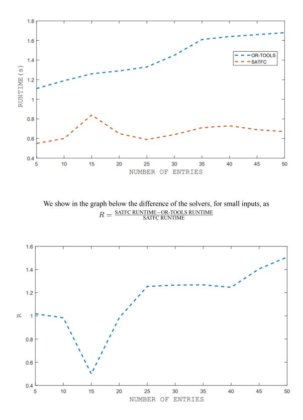
We first show in the graph below the two solvers tested with small size inputs.
