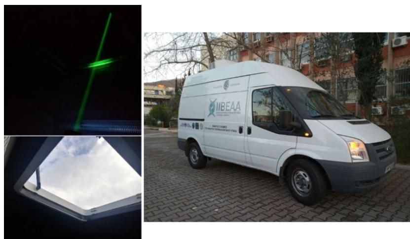
Figure 3.9: The van-mounted 532 nm depolarization AIAS mobile lidar system.
