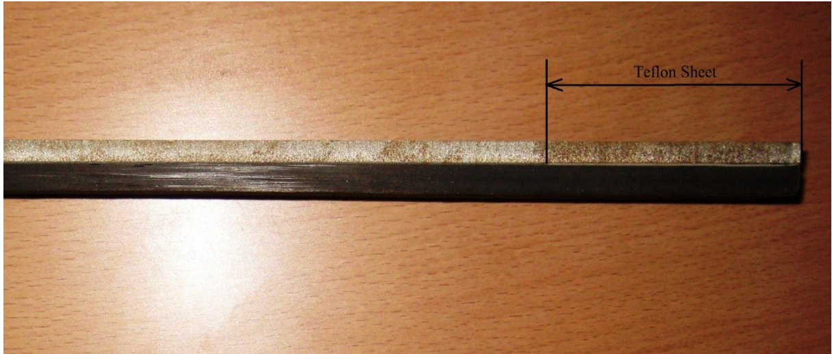
Figure 2.5. A DCB-UBM specimen that was tested in this study. The Teflon sheet used as the initial crack can be seen.
