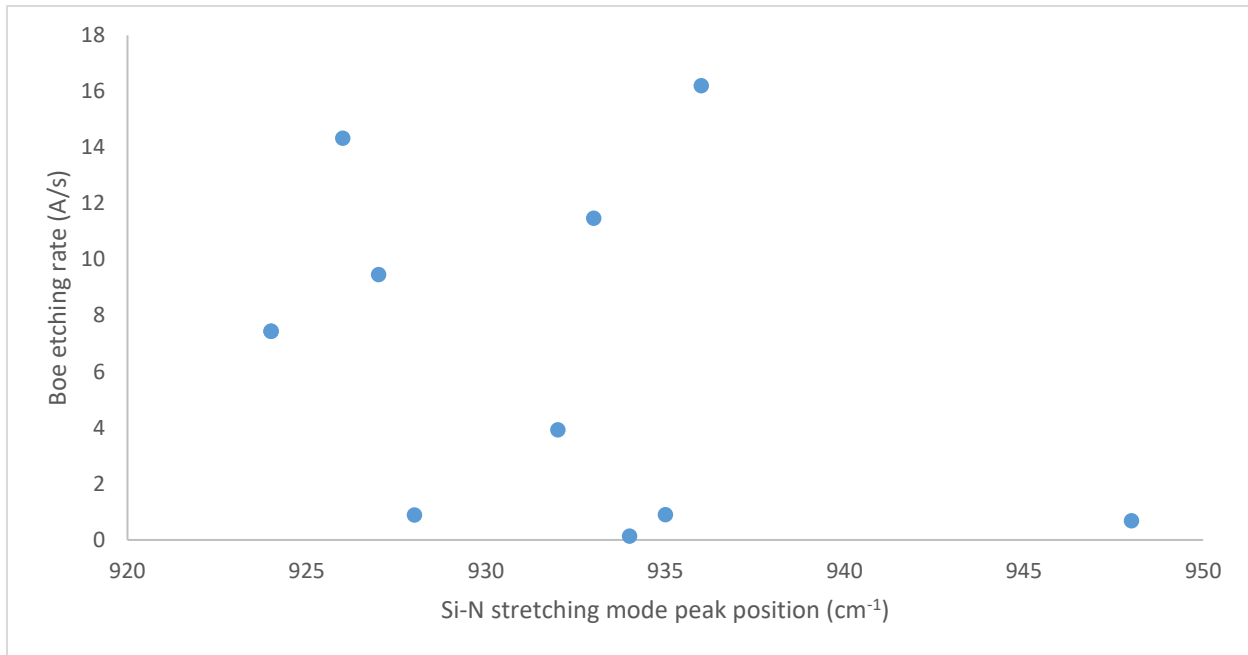
Figure 51: Effect of the Si-N stretching mode peak position on the observed etching rate.
