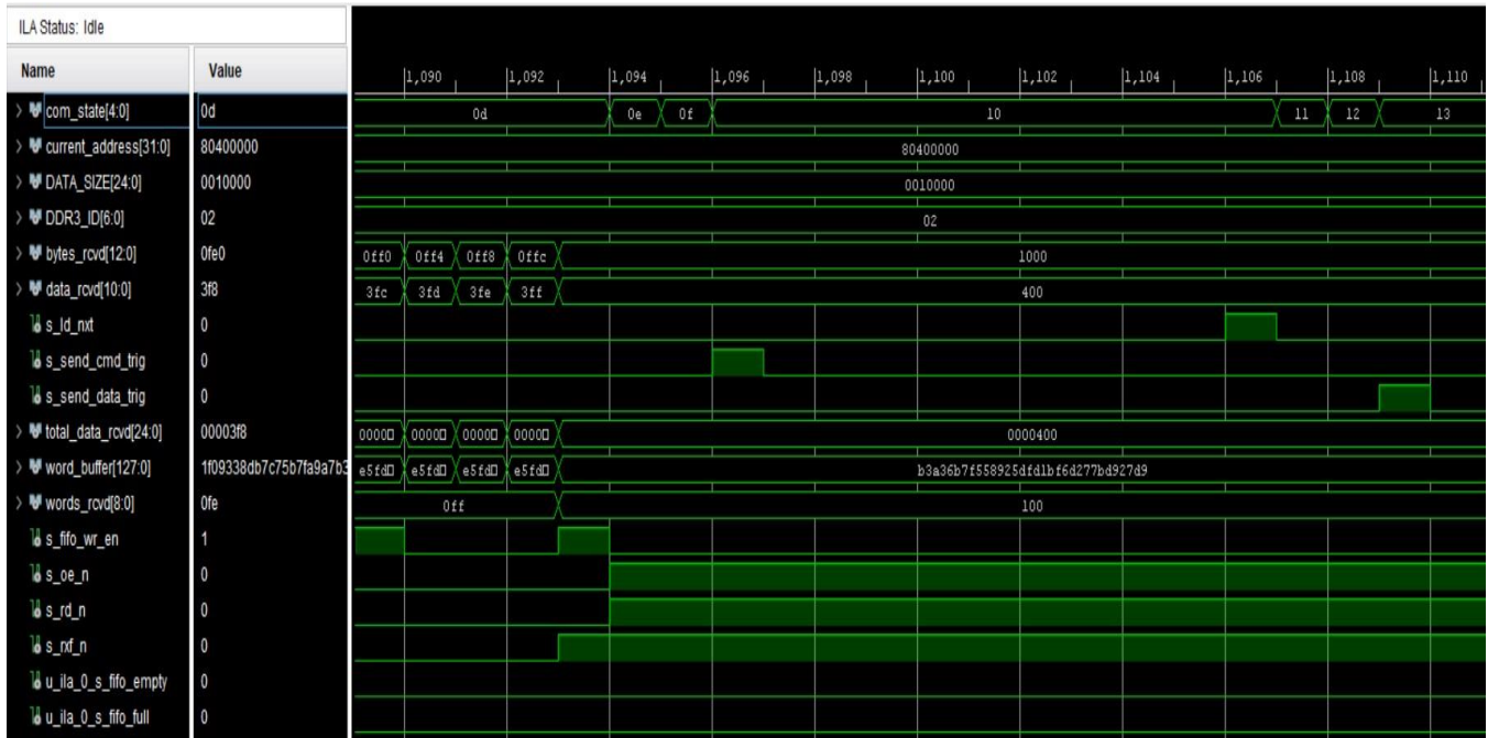
Figure 28: USB3.0 waveform data packet receiving - completion
