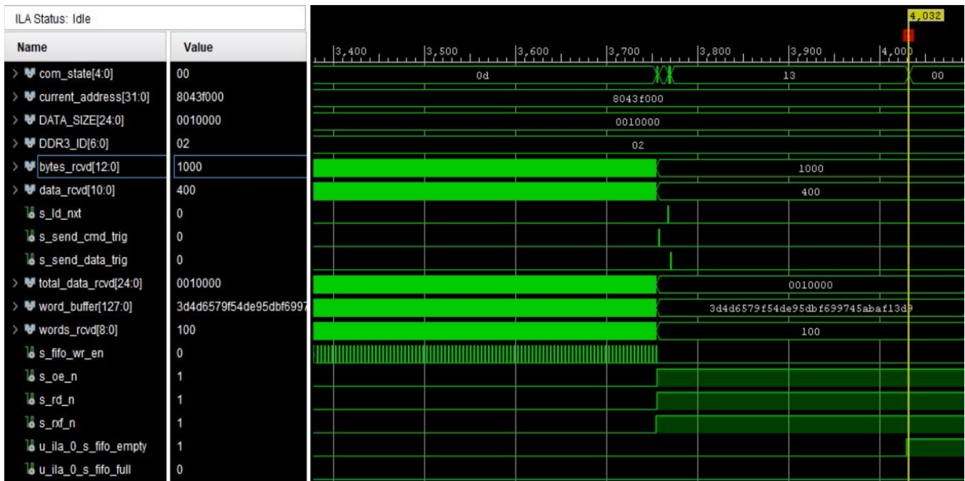
Figure 29: USB3.0 waveform signal receiving - completion
