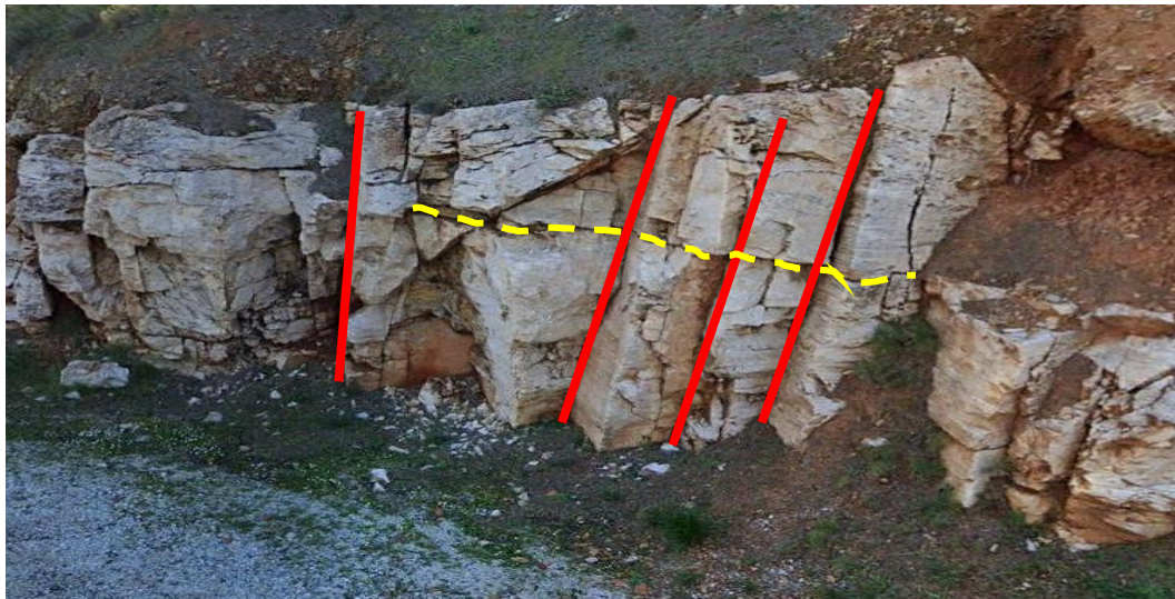
Figure 4: Measurements taken from field, that combine fracture planes of low and high angle slope.
