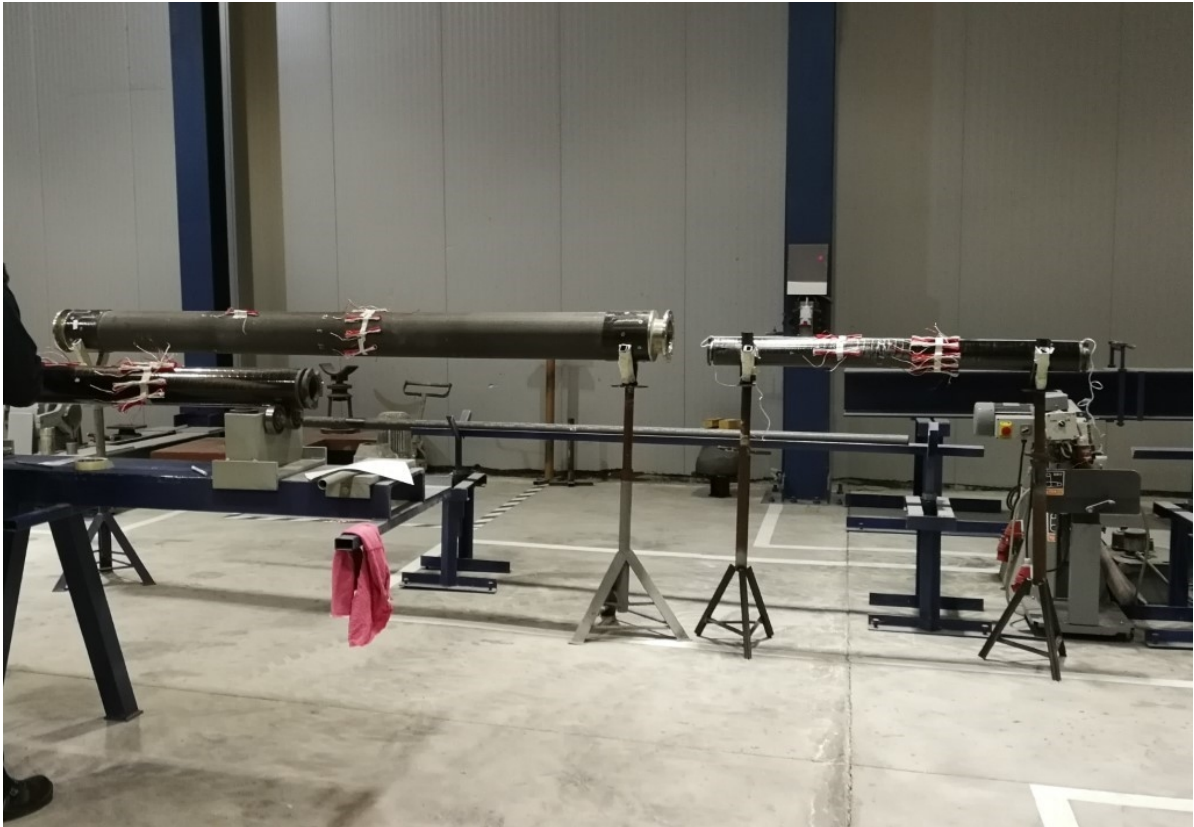
Figure 3.5: Installation of strain gages on the shafts
