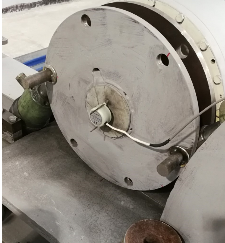
Figure 3.3: Angle measuring sensor (clinometer)
