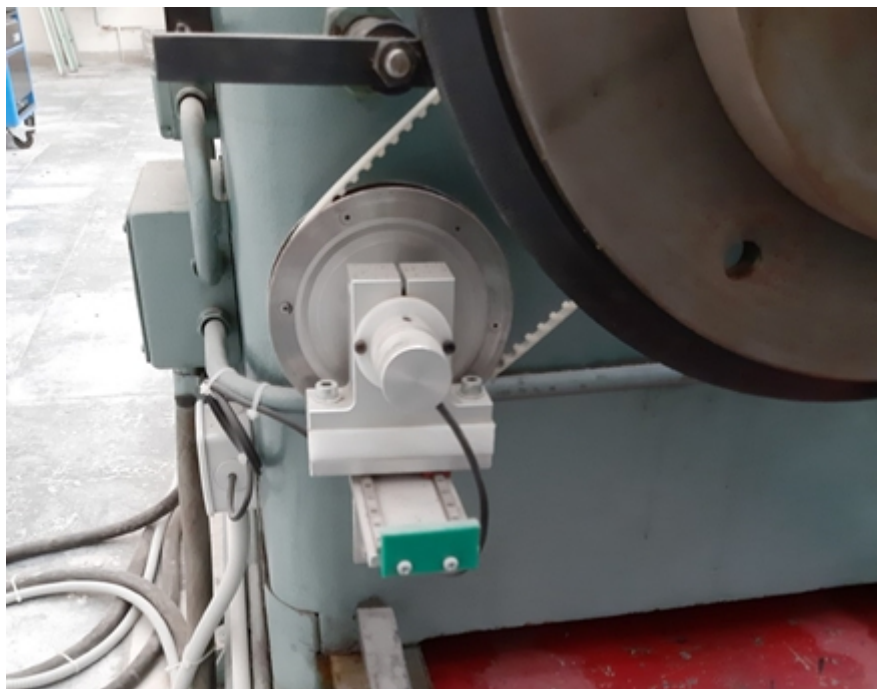
Figure 2.7: Digital clinometer (angle measurement)
