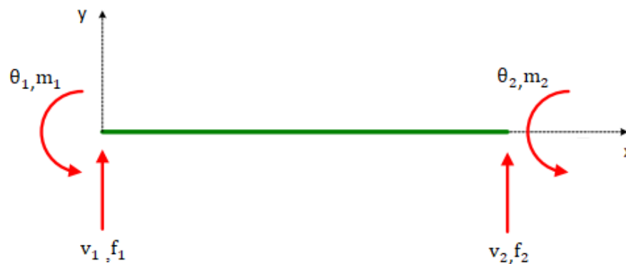
Figure 2.12: Beam with four degrees of freedom
