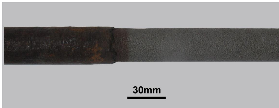
Figure 3.1: Morphology of bare surfaced rod after one year's exposure at splash zone, left is the upper half without removal of rust; right is the lower half, with rust removed.
