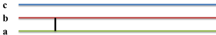
Figure B.3: A line-to-line fault
