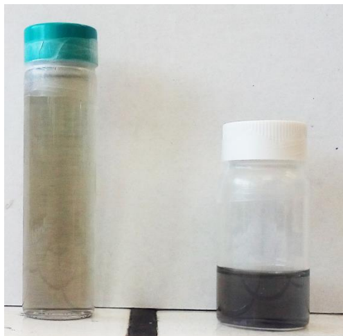
Figure 5.22 Optical images of rGO dispersions in ethanol (left) and DMF (right), two weeks after their preparation. The vial with DMF is half-full.
