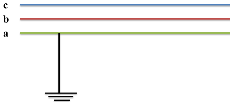
Figure B.1: A single line-to-ground fault
