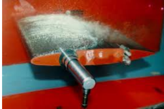
Figure 1.1: Sheet cavitation, taken from https://cavity.caee.utexas.edu
