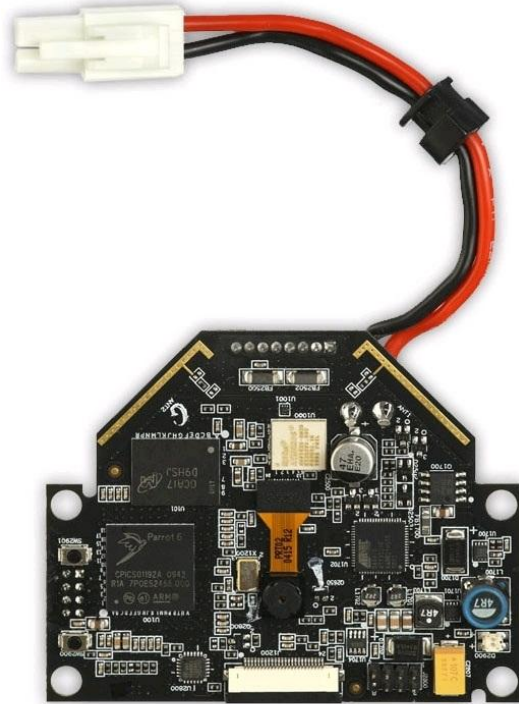
Figure 12 AR Drone Main Board and Downlooking Camera
