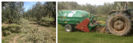
Figure 2: Left: Alignment of olive tree prunings before harvesting; Right: FACMA Comby TR200 harvester used in the demonstration
