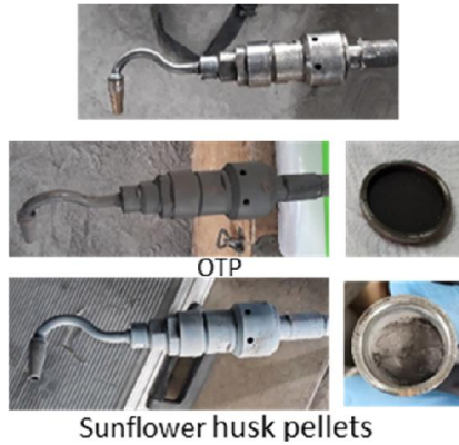
Fig. 2. Nozzle before (top) and after the measurements and the respective filters (right)
