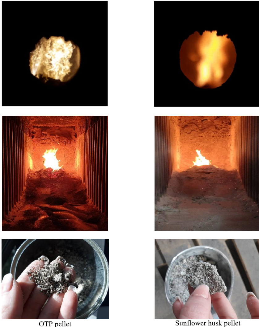
Fig. 4. Combustion of OTP pellets (left) vs sunflower husk pellets (right) at industrial boiler: flame inspection (first row), combustion chamber inspection (second row) and ash formation inspection (third row)
