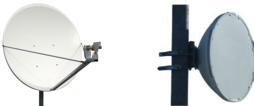
Figure 4-5: The antennas used: 1.2m Ka-band (on the left), 0.6m Q-band (on the right)
