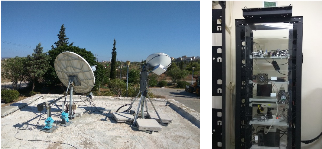
Figure 4-26: Overview of the RF front- and back-end along with all electronic equipment, located at NTUA LTCP.
