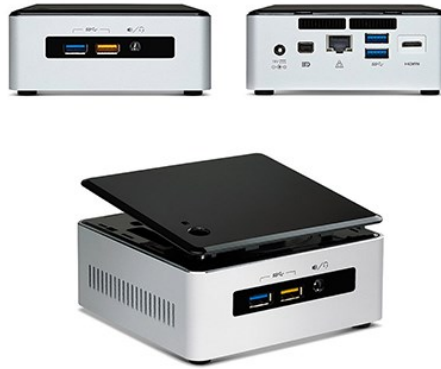
Figure 4-13: The Intel NUC mini-computer currently used at each location.
