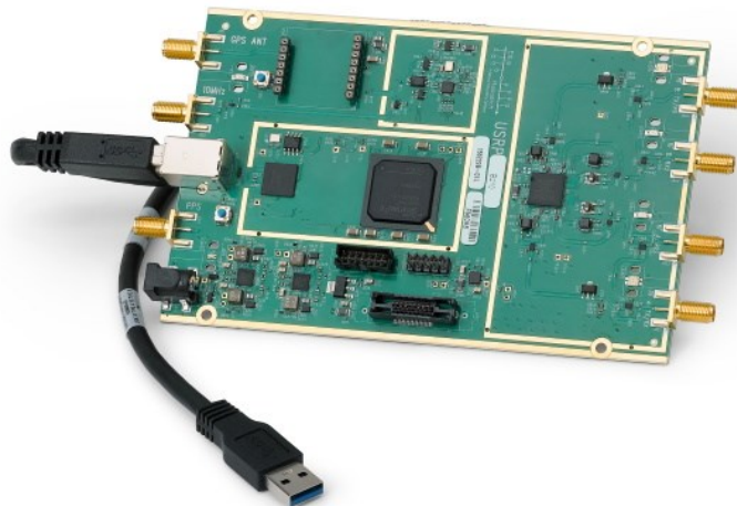
Figure 4-11: The Ettus USRP B210 SDR device used
