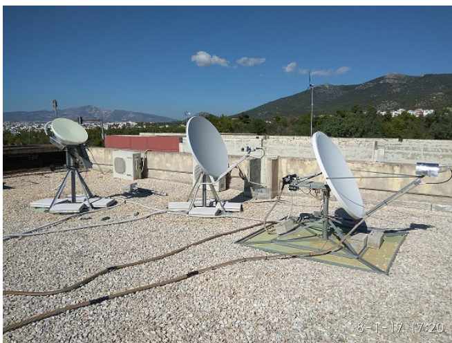
Figure 4-25: Overview of the RF front- and back-end along with all electronic equipment (outdoor enclosure), located at NTUA Campus.
