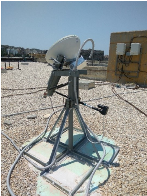
Figure 4-24: Overview of the Q-band front-end installed at NTUA Campus (on the left) and NTUA LTCP (on the right)
