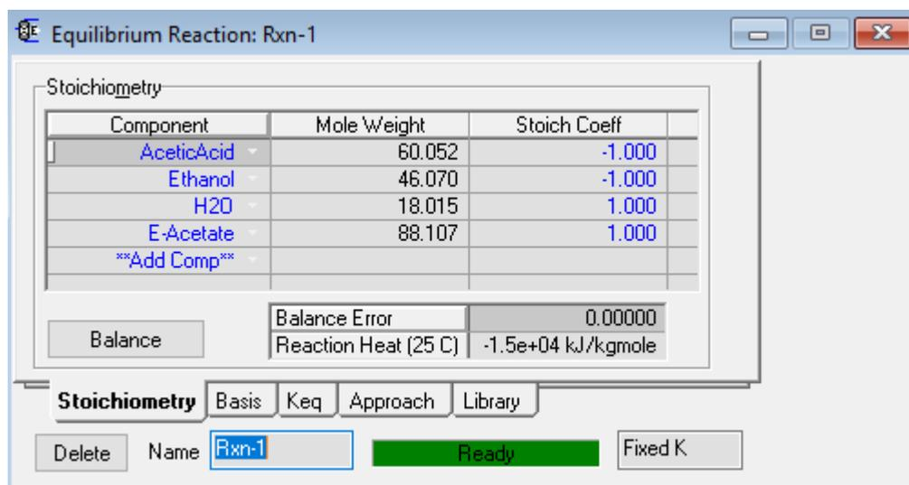
Figure 10.9. Inserting components and stoichiometric coefficients for a reaction in UniSim.
