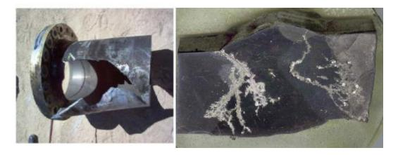
**Figure 2.1.** Left image: A ruptured heat exchanger inlet nozzle due to mercury corrosion [11]; right image: Mercury-induced liquid metal embrittlement on a brazed aluminum heat exchanger [12].
