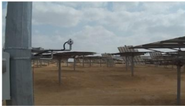
Figure 1-21. A patented instrument that can measure global and diffused insolation. 4 SPN1 instruments are installed, in the 4 corners of the perimeter of the solar field (Minis et al., 2019) [32]
