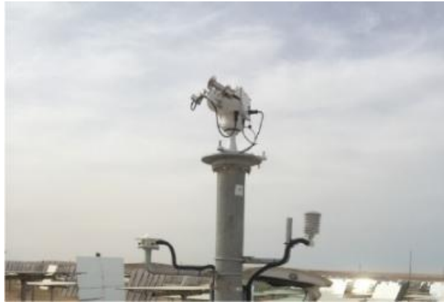
Figure 1-19. Epply Model sNIP Pyrheliometer in Ashalim (Minis et al., 2019) (Minis et al., 2019) [32]
