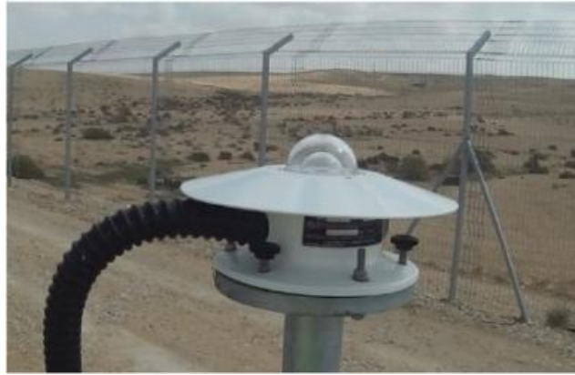
Figure 1-20. Pyranometer, used to measure the global irradiance, leveled on a horizontal plane in Ashalim (Minis et al., 2019) [32]
