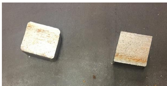
Figure 4.5: S700 after cutting with discotom.
