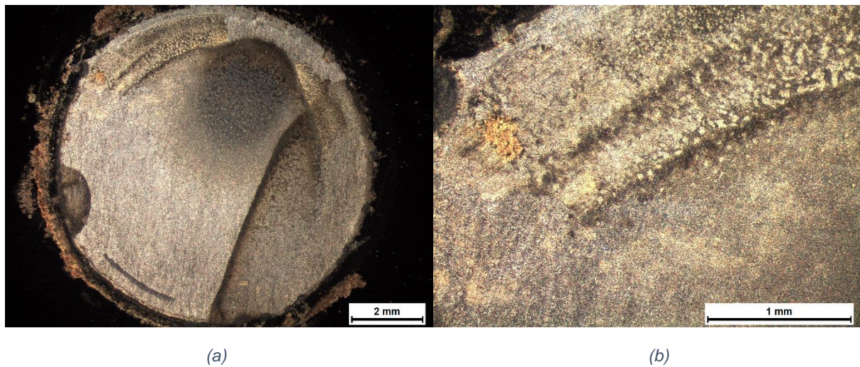
Figure A.1: Optical observation of S560 after 24hour experiment on Open Circuit method. Stereomicroscope's magnification at (a) x1.0, (b) x4.0
