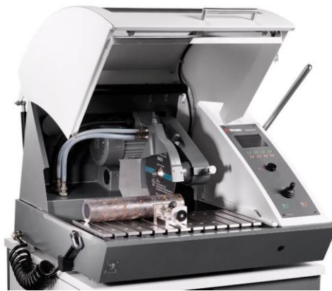
Figure 4.4: Struers discotom of STL [ www.struers.com ].
