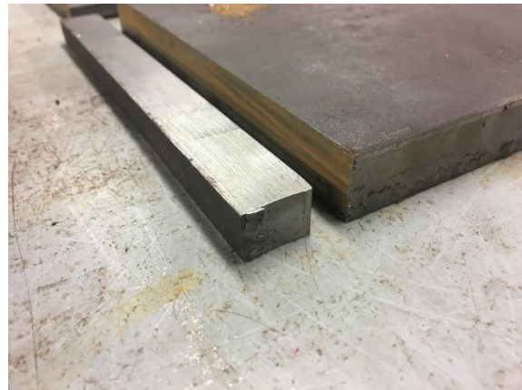
Figure 4.3: S700 after cutting with band saw.
