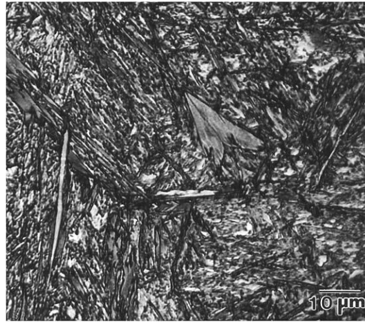
Figure 1.3: Martensite (A fully martensitic microstructure. Sodium metabisulfite etch. 1000x). [Bramfitt and Benscoter, 2002]
