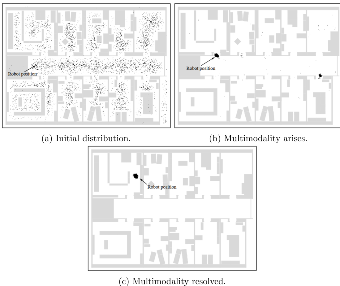
Figure 2.5: Particle filter iterations. Initially, the robot is highly uncertain of its whereabouts. Then, two highly likely locations are determined based on observations. Moving to collect more data, the robot finally localizes itself. [5]
