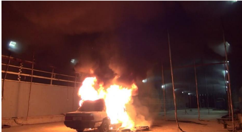
Figure 3.1. A vehicle fire test in an Immersed Model Tunnel, China (Xu et al. 2018).
