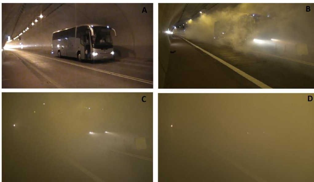
Figure 3.10. Visibility Levels during an evacuation Experiment in "Emilia" Tunnel, Poland, 2016.
