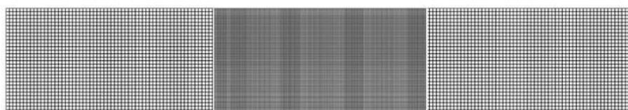
Figure 3.11. A representation of a refined grid resolution at the fire region, at YingZuiYan Road Tunnel simulation (Hu et al., 2010)
