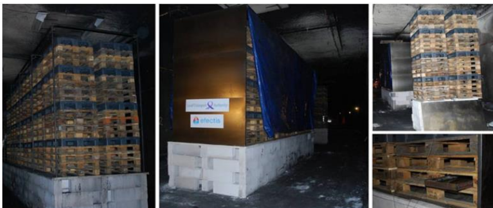
Figure 3.3. A simulated HGV, consisting of wooden & plastic pallets, utilized in San Pedro Tunnel Fire Experiment, Spain (Cheong et al., 2014).
