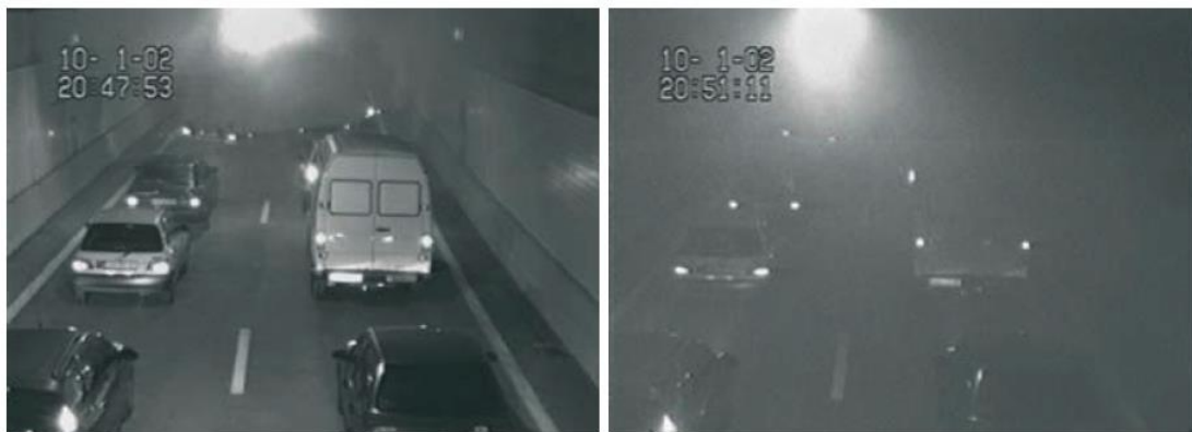
Figure 3.8. Flashing Alarm Lights In Traffic Congestion In Benelux Tunnel Evacuation Experiment, 2005.
