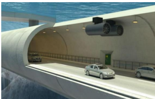
Figure 2.7. Future project of submerged floating tunnels in Western Norway ( https://www.ctif.org/news/explosions-fire-and-overload-biggest-challenges-norway-builds-worlds-first-floating-tunnel ).
