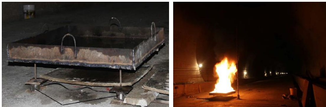
Figure 3.4. Weighing system of a fuel pool, in Baimang Snow Mountain No.1 Tunnel Experiment, China (Yan et al. 2017).
