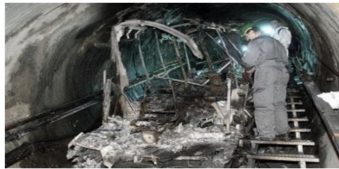
Figure 2.6 Picture of a funicular railway incident, in the Austrian Alps, where more than 150 people have lost their lives in an intense fire, in 2000.
