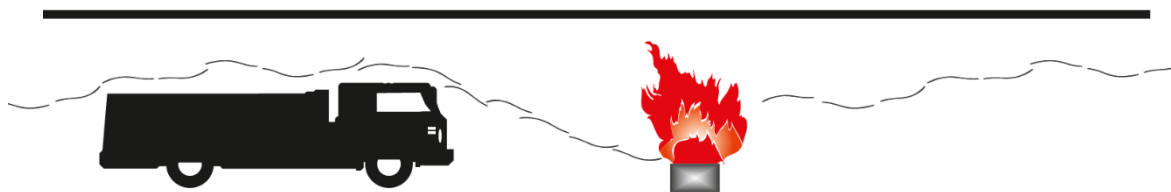
Figure 2.16. A schematic diagram of a blockage existence near the fire source along with the resulting smoke spreading upstream and downstream from the fire.
