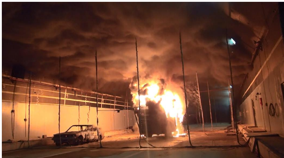
Figure 3.6. Smoke stratification and propagation, during a vehicle fire, (Xu et al. 2018).
