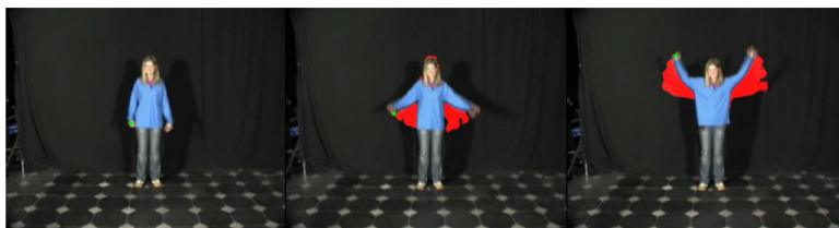
Figure 3.2: A measure of QoM using SMIs (the shadow along the arms and the body) and the tracking of the hand. Source: [18].
