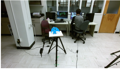
Figure 8.12 (a) Demonstration of an “Observed” RGB frame of the “Stability far” scenario with a rendered predicted pose of the “Dragon” model, generated by the baseline tracker of Garon et al.[83].
