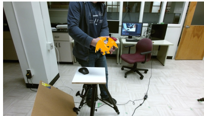
Figure 8.55 (b) Demonstration of an “Observed” RGB frame of the “Hard Interaction” scenario with a render predicted pose of the model generated by the baseline tracker of Garon et al.[83] with Residual inter-layer connections and augmentation/initialization/sampling strategic improvements.
