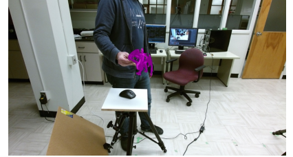
Figure 8.35 (c) Demonstration of an “Observed” RGB frame of the “Translation Only Interaction” scenario with a render predicted pose of the model generated by the proposed tracker.
