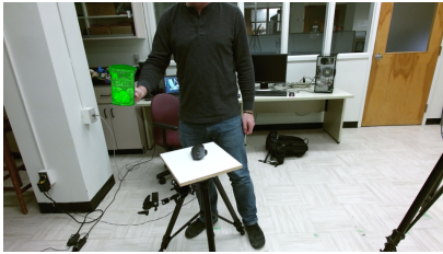
Figure 8.141 (d) Demonstration of an “Observed” RGB frame of the “Translation Only Interaction” scenario with a rendered predicted pose of the “Cookie Jar” model generated by proposed tracker, with the special case of unique rotational symmetry parameter, that remains frozen after training, of this work.
