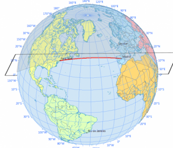
Figure 3.53 The Geodesic (shortest) distance path, on the globe, which is created by the intersection of the globe with the greatest plane passing from the 2 points of the globe and at a direction that follows the globe's parallels.
