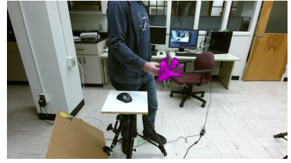
Figure 8.49 (c) Demonstration of an “Observed” RGB frame of the "Full Interaction" scenario with a render predicted pose of the model generated by the proposed my tracker.
