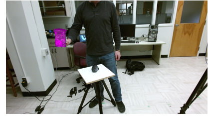
Figure 8.140 (c) Demonstration of an “Observed” RGB frame of the “Translation Only Interaction” scenario with a rendered predicted pose of the “Cookie Jar” model generated by proposed tracker of this work.
