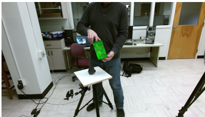
Figure 8.160 (d) Demonstration of an “Observed” RGB frame of the “Rotation Only Interaction” scenario with a rendered predicted pose of the “Cookie Jar” model generated by proposed tracker, with the special case of unique rotational symmetry parameter, that remains frozen after training, of this work.
