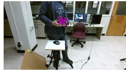
Figure 8.42 (c) Demonstration of an “Observed” RGB frame of the “Rotation Only Interaction” scenario with a render predicted pose of the model generated by the proposed tracker.
