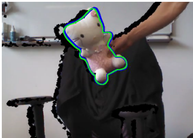
Figure 2.3: Per-frame Object 6D Pose Detection based on Learning to Regress Object Coordinates. [8]
