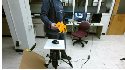
Figure 8.34 (b) Demonstration of an “Observed” RGB frame of the “Translation Only Interaction” scenario with a render predicted pose of the model generated by the baseline tracker of Garon et al.[83] with Residual inter-layer connections and augmentation/initialization/sampling strategic improvements.
