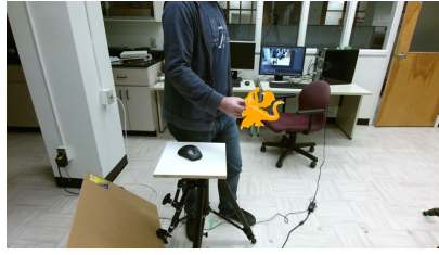
Figure 8.48 (b) Demonstration of an “Observed” RGB frame of the "Full Interaction" scenario with a render predicted pose of the model generated by the baseline tracker of Garon et al.[83] with Residual inter-layer connections and augmentation/initialization/sampling strategic improvements.
