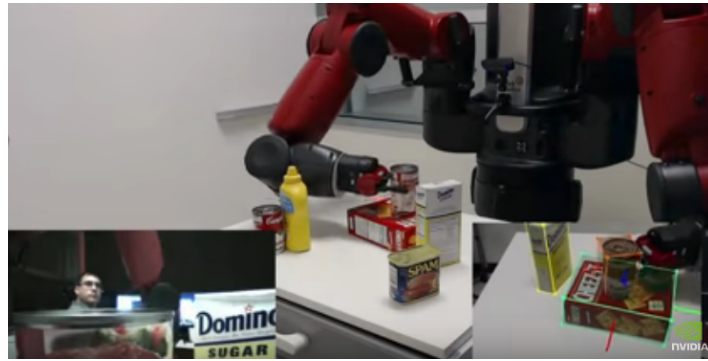
Figure 10.16: Overview of an example of using 6D Pose Estimation as a prior for successful household object grasping. Grasp hypotheses are generated, based on the Object Pose estimations, and they are verified or discarded at a later, cascaded level [137].
