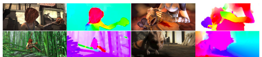
Figure 3.4: Dense Optical Flow examples given by the FlowNet2 architecture in the synthetic 'Sintel' video dataset.[52]
