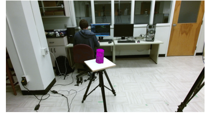
Figure 8.83 (c) Demonstration of an “Observed” RGB frame of the “Stability far” scenario with a rendered predicted pose of the “Cookie Jar” model generated by proposed tracker of this work.
