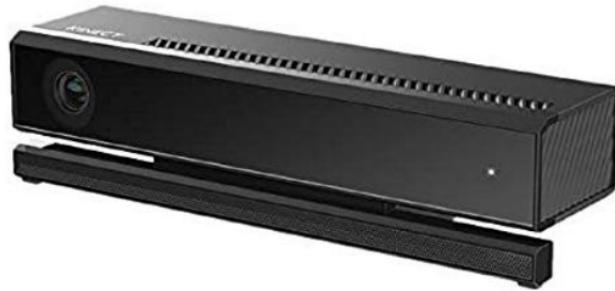
Figure 2.2: The second and most recent version of the Microsoft Kinect RGB-D sensor.
