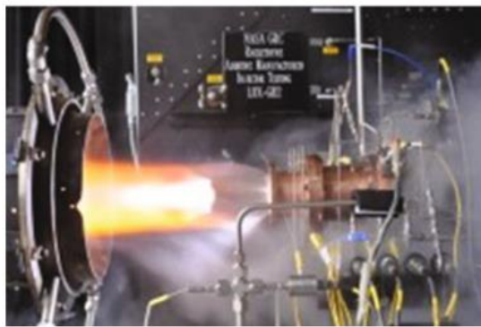
Fig. 1.42 Testing of an additive manufactured rocket nozzle.
