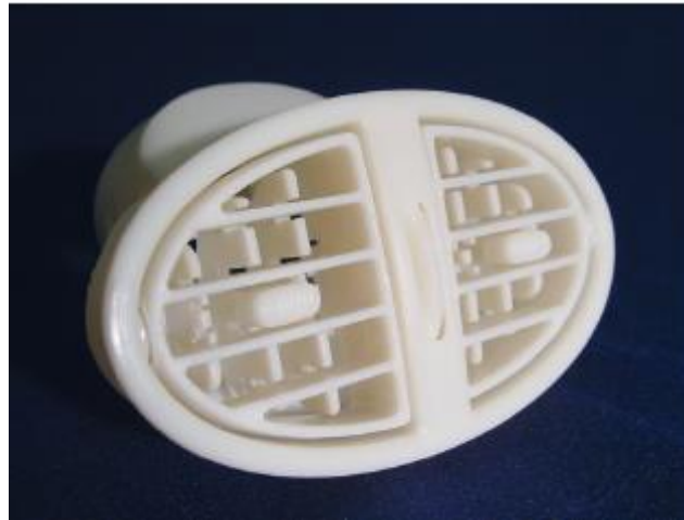
Fig. 1.3 Functional prototyping: adjustable air-outlet grille for a passenger car; laser stereolithography.
