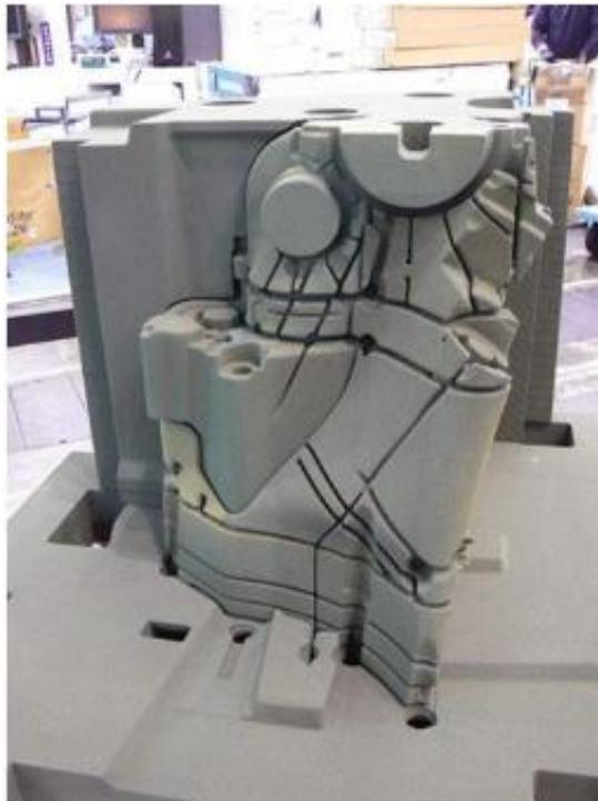
Fig. 1.46 Binder Jet produced silica sand mold for casting an aluminum Formula 1 transmission housing.
