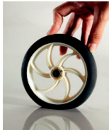
Fig. 1.11 Polymer jetting: structure (left); two-material wheel with elastic tire (right).
