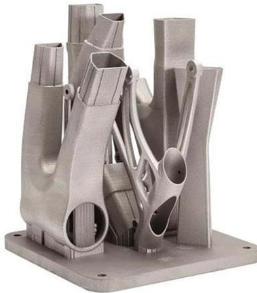
Fig. 1.34 Titanium bike frame as-built using AM.
