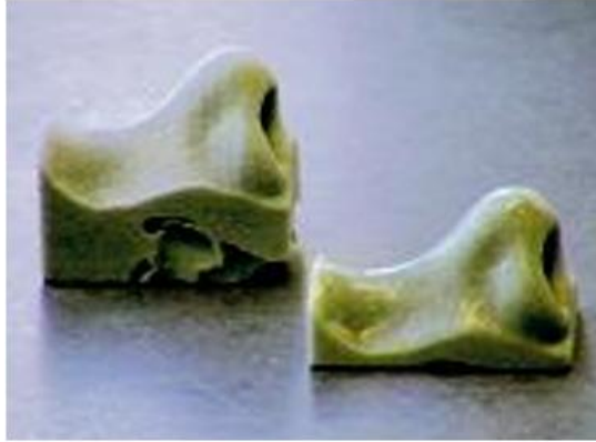
Fig. 1.21 Powder-binder process; improved surface quality by manual finishing: part as from the machine (left) and after finishing (right).
