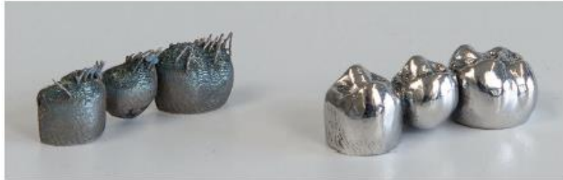
Fig. 1.4 Direct manufacturing: dental bridge (three elements directly after manufacturing; without removing of support structure (left), after finishing (right); selective laser melting (SLM), CoCr alloy.
