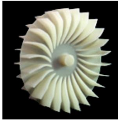
Fig. 1.26 Layer laminate manufacturing; plastic laminate printers; machine (left); fan wheel made by the laminate Printer Solido SD 300 pro, PVC (right).
