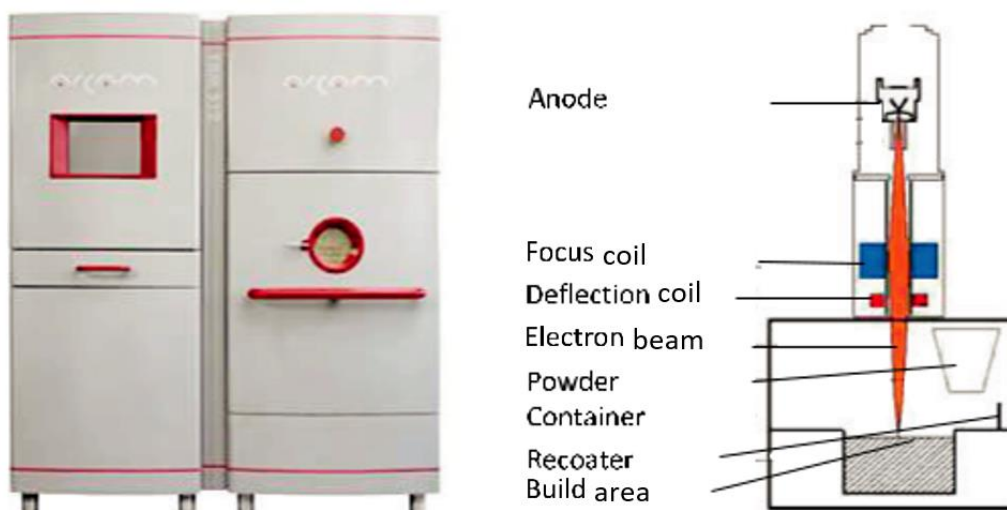
Fig. 1.18 Electron beam melting (EBM): EBM System A2 (left); EBM scheme (right).
