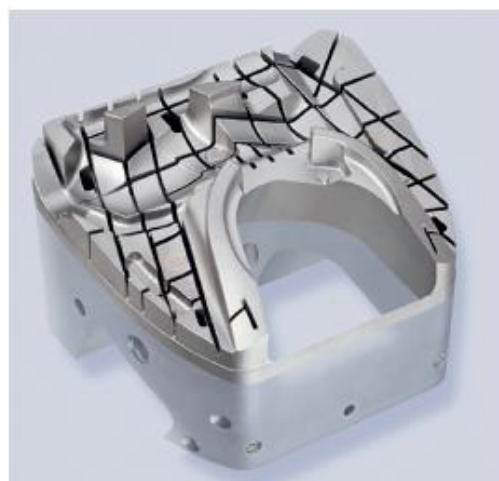
Fig. 1.5 Direct tooling: mold insert with conformal cooling channels (dark) and pneumatic ejectors (white); laser sintering/ laser melting; tool steel.
