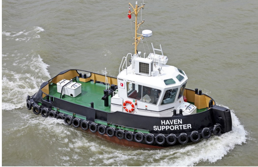
Figure 4-2: The tug vessel considered in this work, model DAMEN Stun Tug 1205 from Damen Shipyards Group (NL), L = 13.8 \text{ m} , \Delta = 58 \text{ t} .
