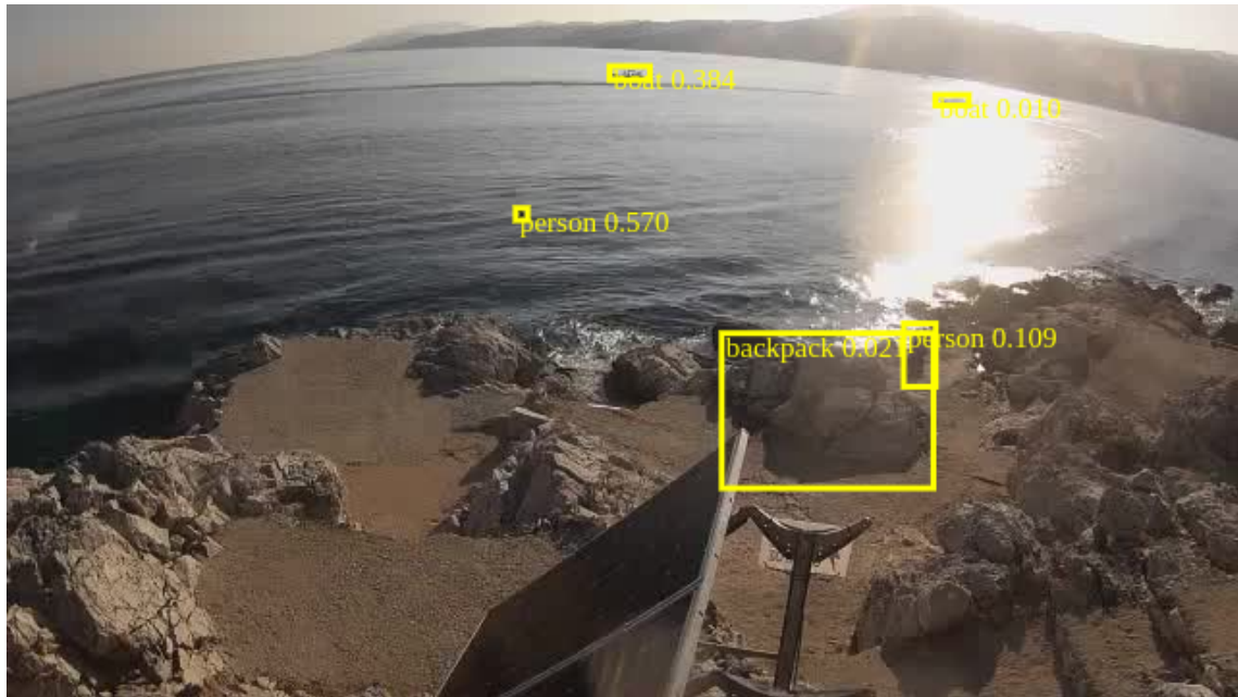
Figure 4.10: Predictions of standard YOLOv3 on lowered score threshold with one vessel in not ideal lighting conditions.
