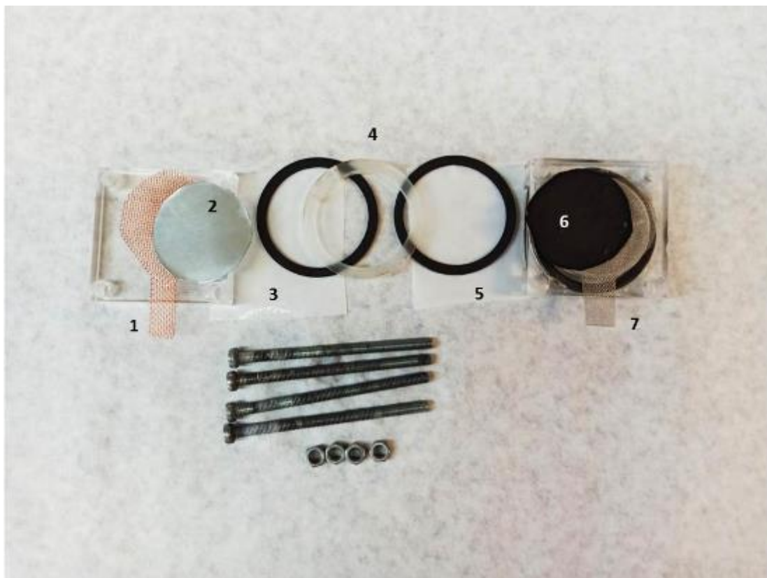
Figure 11: Assembling sequence of components in zinc-air cell; (1) Cu Mesh/ Current Collector (2) Zinc polished plate / Anode (3),(5) Separator Membrane (4) Electrolyte entrance (6) Coated CP/ Cathode (7) Ni Mesh/ Current Collector
